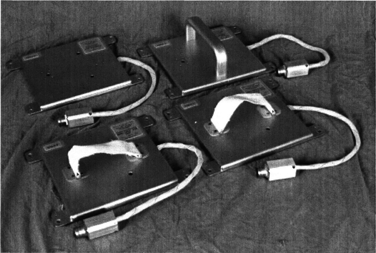
Figure 4.8: The photograph shows the four EDLS sensors: one touchpad, one handhold, and two foot restraints (NASA Image JSC S95 17030).
