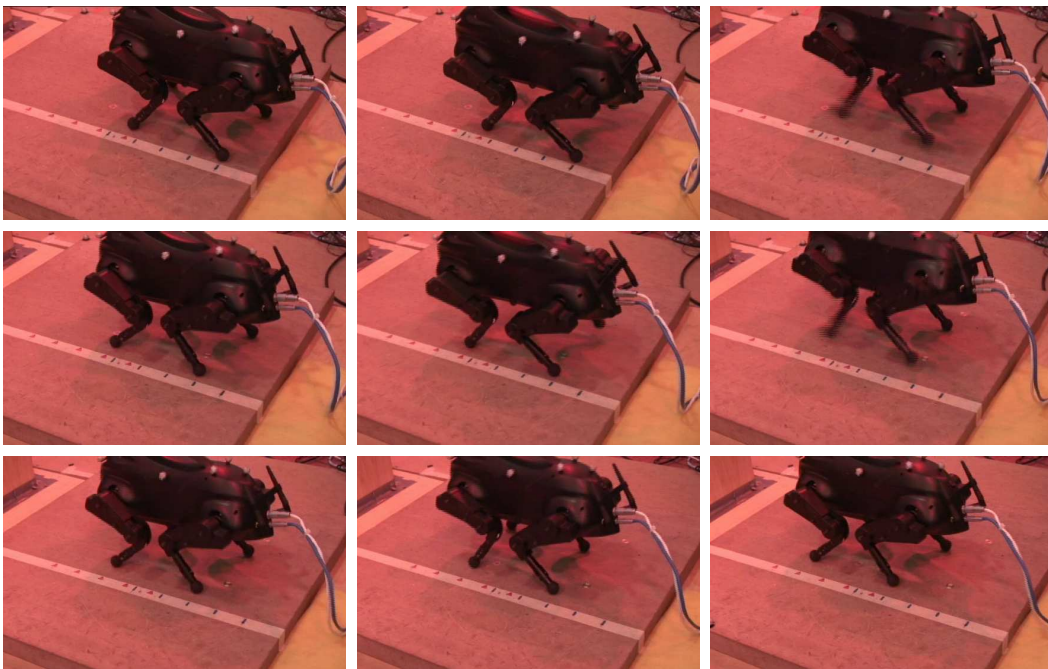
Figure 3-21: Demonstration of accuracy in positioning pacing steps. The rear left foot should align with the black circle marks and the front left foot should align with the red triangles. Spacing between consecutive circles (and triangles) is 4 cm. Pacing steps of up to 10 cm can be achieved to create continuous, forward locomotion.
