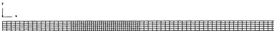
Figure 4.8: Finite Element Mesh of the Top View of Cantilevered, Steel Beam with Rectangular Actuator
