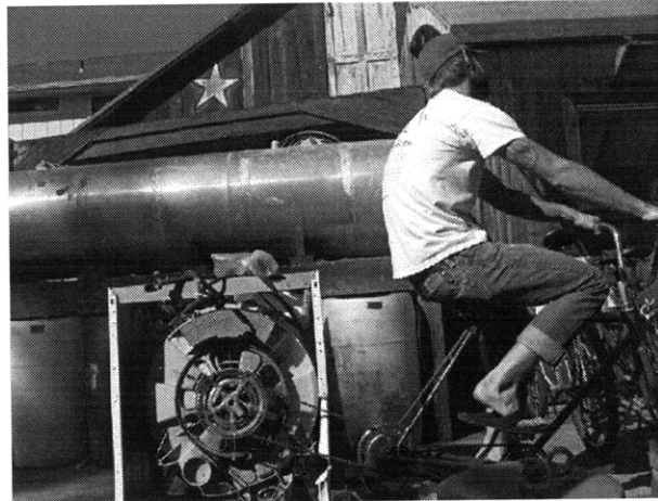
(b) front-loading washer direct chain drive (source: http://www.appropedia.org )
