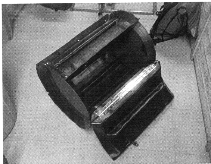
Figure 5-6: Side-loaded, multi-part, structural drum prototype
