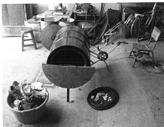
(b) design built at Maya Pedal using a 34 gal plastic barrel
