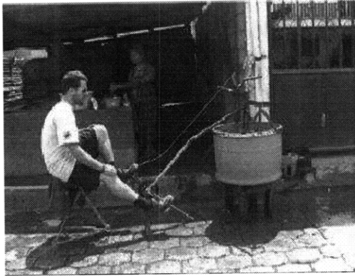
(a) machine is actuated by strings tied to the end of the pedals
