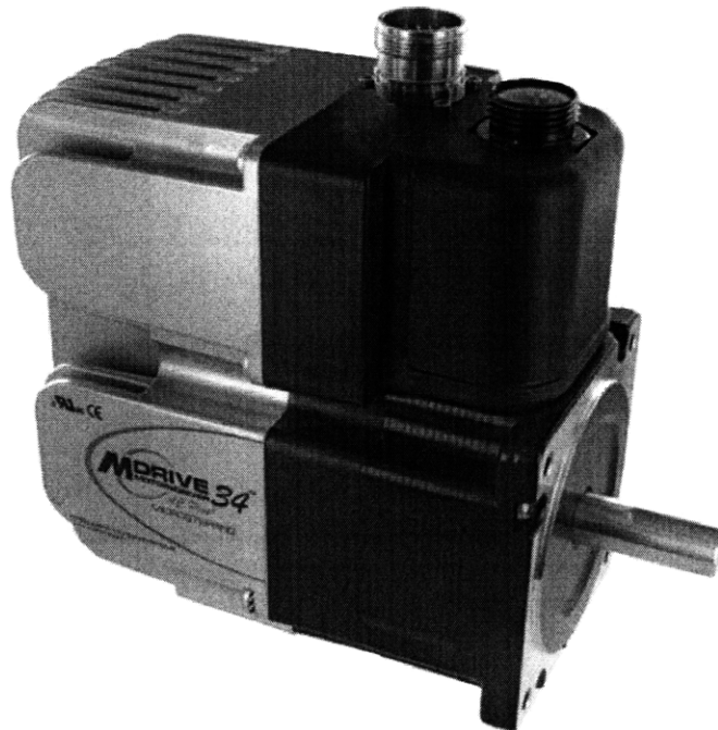
Figure 5-10 The IMS NEMA 34 stepper motor with integrated power supply and driver was used to drive the print roller, drive roller, and collect roller. This model only required the user to attach 120VAC power and IO; both which were supplied via cables from the manufacturer.
