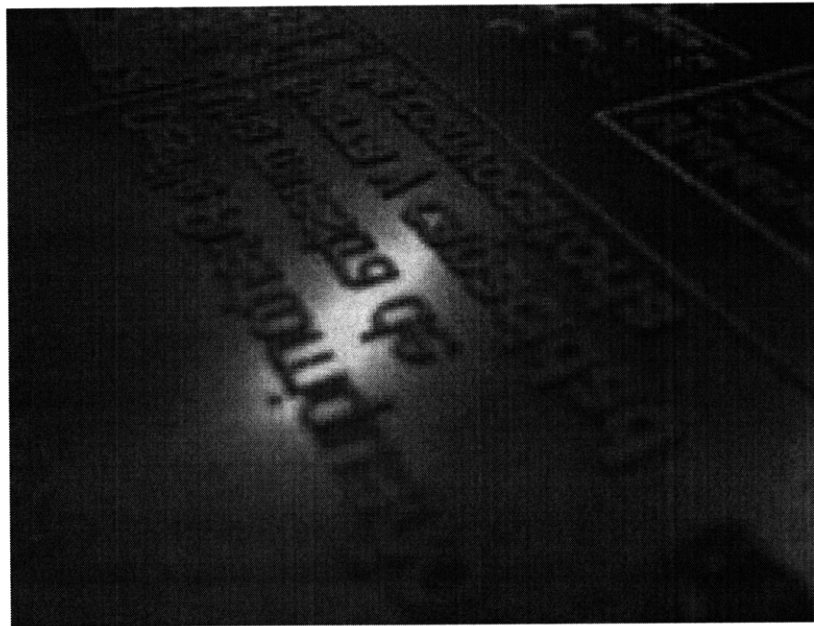
Figure 3-1: A close-up of a relief stamp used in flexographic printing [17]
