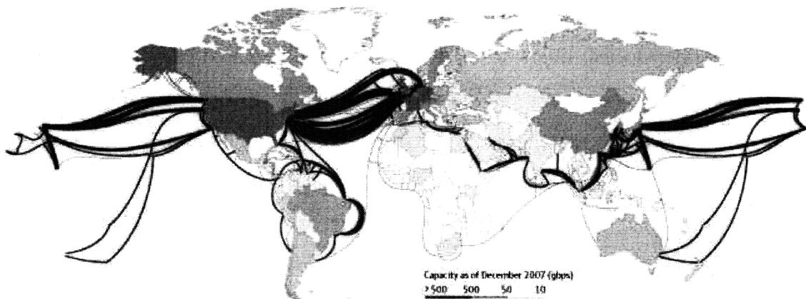
Figure 1-2: Map of transcontinental fiber-optic submarine cables [1]
