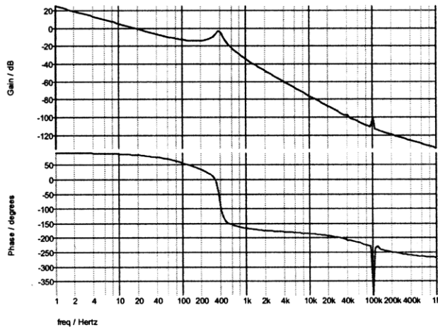
Figure 3-20: Simulated Bode plot of loop gain
