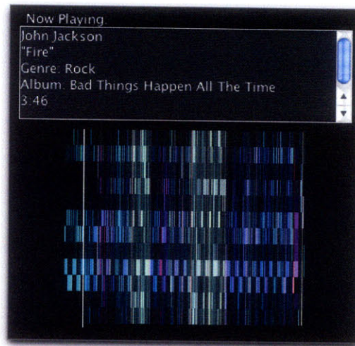
Figure 5-16: Song information. Metadata and soundsieve image for the current (or most recent) song are displayed. A white vertical line moves across the soundsieve image during playback, indicating the current location in the song.
