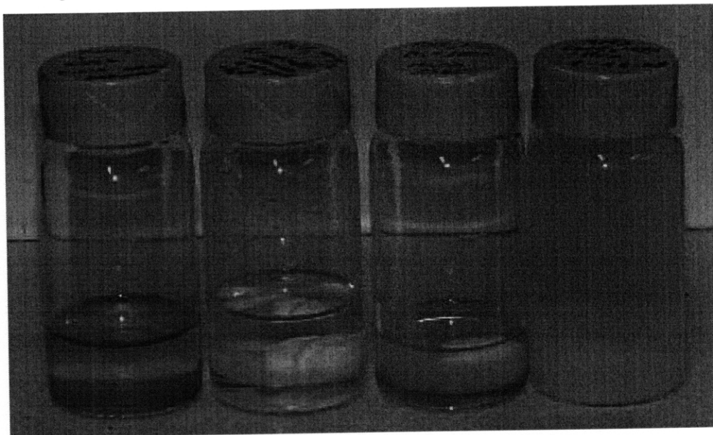
Figure 4 Photograph of vials with different catalyst solutions (from left to right) \text{FeCl}_3 solution, Hexanes/ \text{FeCl}_3 solution before stirring, segregated mixture, stable mixture
