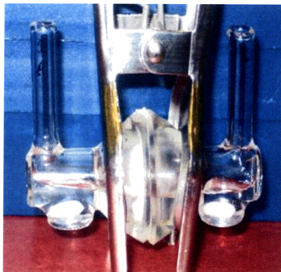
Figure 3-3. Side-by-side diffusion cell used to quantify analyte diffusion. The membrane is clamped between the two glass chambers. A radiolabeled solution is added to one chamber and at each time point a small volume of liquid is removed from the other chamber to quantify the amount of radioactive material that has diffused across the membrane. In this experimental set-up, all the time points are taken using the same membrane.
