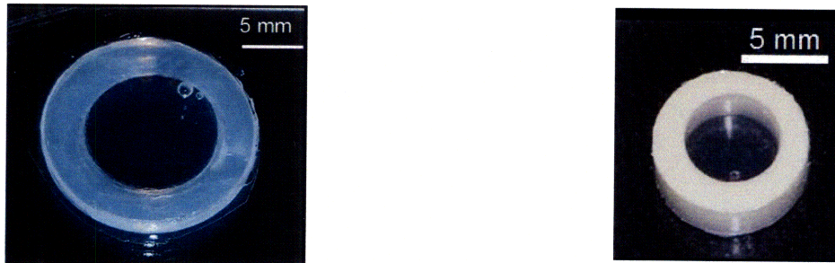
Figure 2-3. Washer devices used for in vitro leak tests and sensing experiments. The device on the left is an LDPE substrate and uses a silicone adhesive to seal the polycarbonate membrane to the device substrate. The device on the right is an HDPE substrate with double-sided pressure sensitive adhesive used to adhere the polycarbonate membrane to the device substrate.
