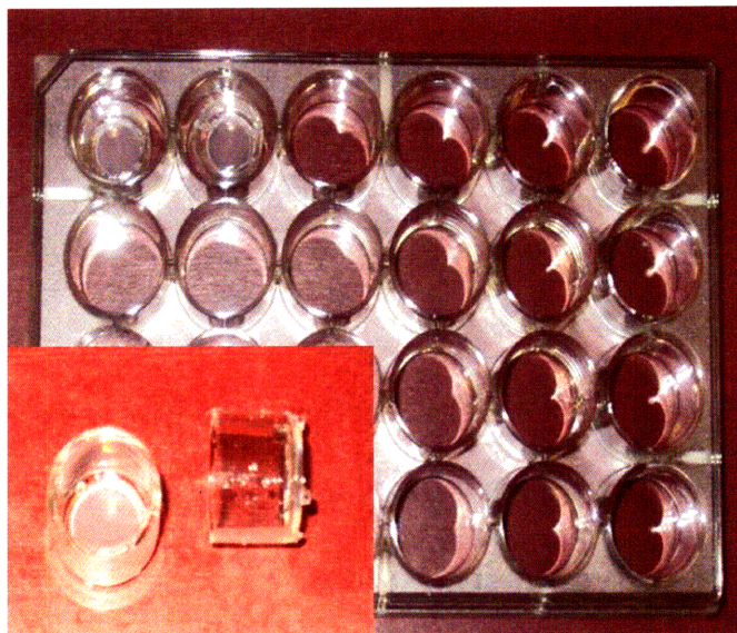
Figure 3-2. 24-well plate format for quantifying analyte diffusion through aluminum oxide membranes. A close-up of the diffusion insert is shown in the bottom left corner. The insert held the radiolabeled analyte solution and the solution in the well of the 24-well plate (receiver solution) was removed at each time point to quantify the amount of radioactivity that had diffuse across the membrane. Each time point in a diffusion experiment came from a different membrane.
