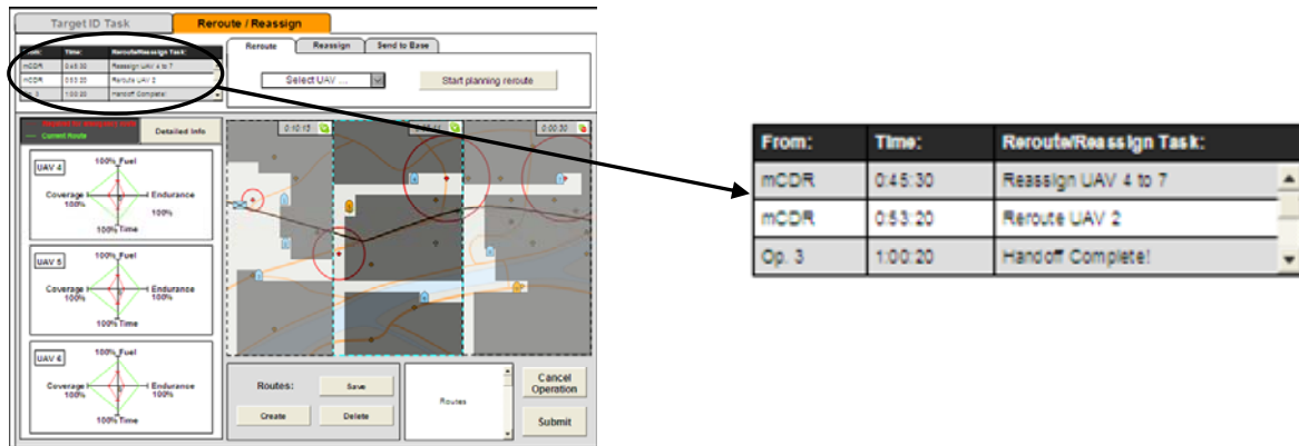
Figure 23. UAV replanning requests in the UAV Replanning panel of the Tasking Display.
