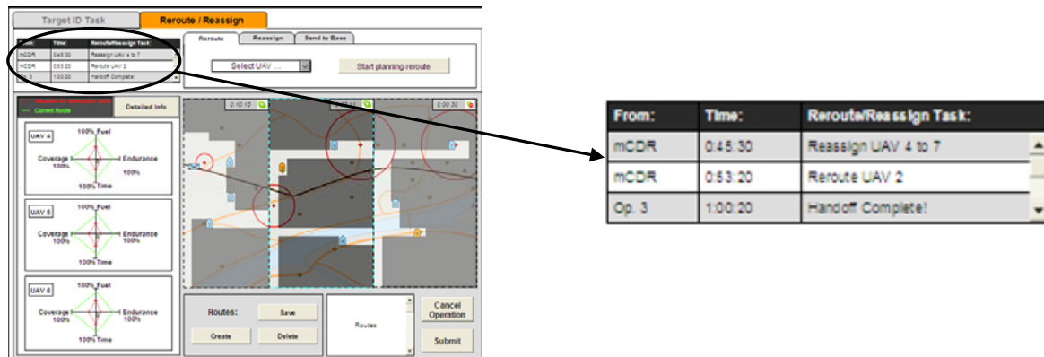
Figure 38. UAV route replanning requests on the UAV Replanning panel of the Tasking Display.
