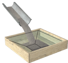
Step Four: Cast Concrete using Plastic Facade Unit
