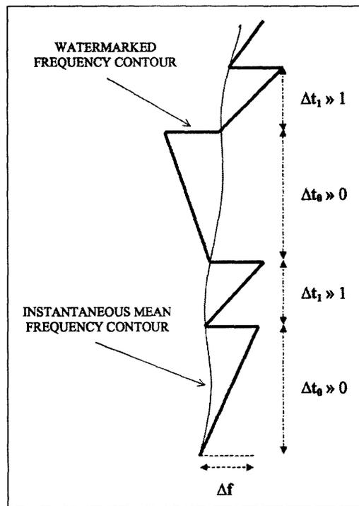
Figure 4-17: Watermarking scheme based on linear chirp segments with abrupt frequency shifts
