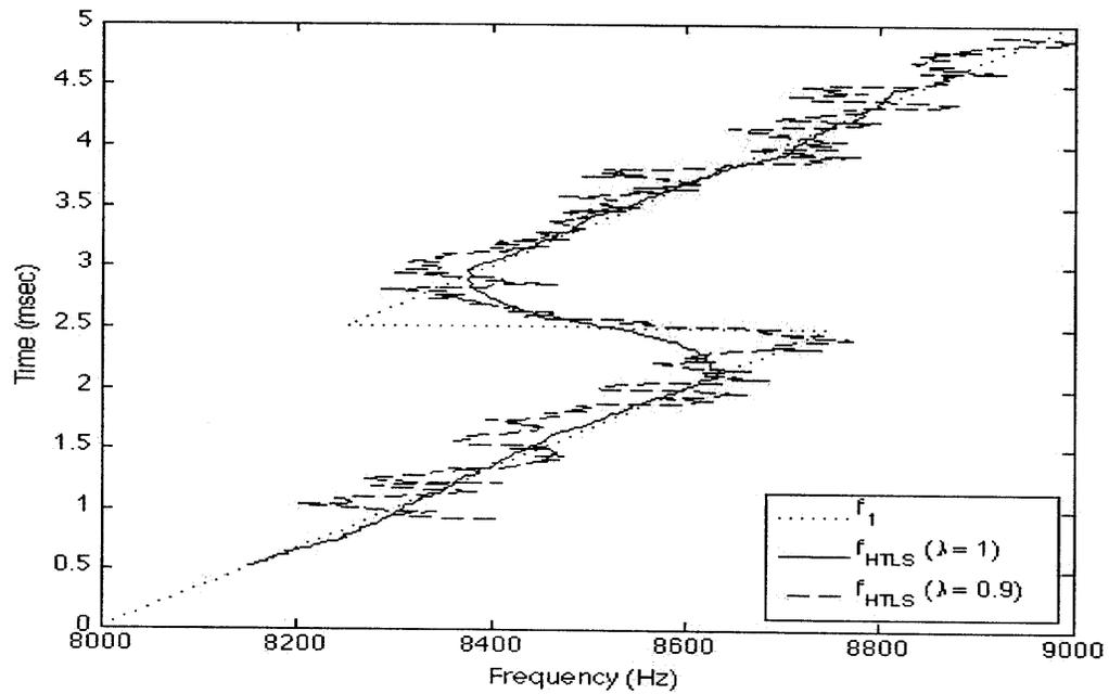
Figure 3-4: HTLS frequency tracking performance vs.  $\lambda$  (SNR = 15 dB)
