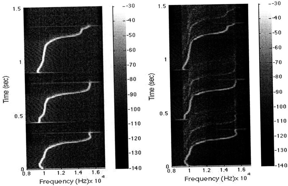
Figure 5-2: Spectrograms of unmodified synthetic whistle calls received at the reference (left) and N1000 (right) hydrophones (dB)
