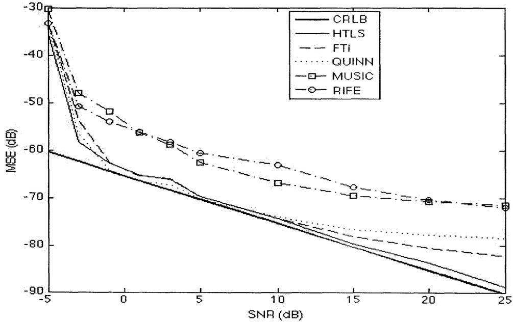
Figure 3-6: Linear chirp frequency estimator performance vs. CRLB
