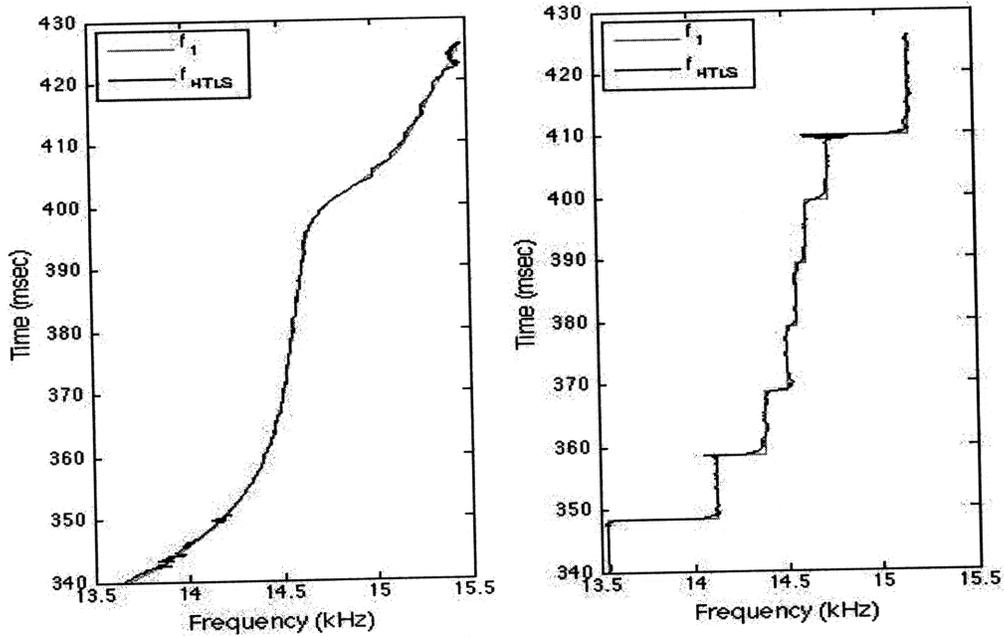
Figure 5-6: Frequency estimation performance for unmodified (left) and watermarked (right) whistle contours received at N1000 hydrophone
