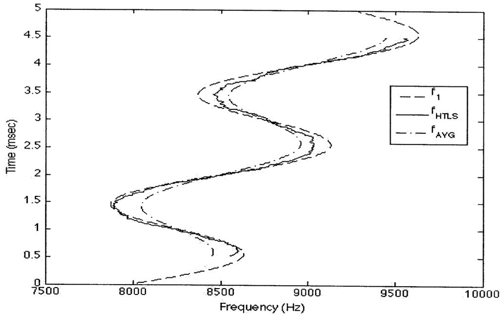
Figure 3-5: HTLS frequency tracking performance for sinusoidal chirp (SNR = 5 dB)
