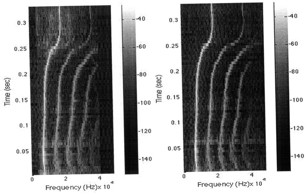
Figure 4-8: Spectrograms of recorded (left) vs. synthetic (right) versions of Whistle 1 in Fig. 4-1 (dB)
