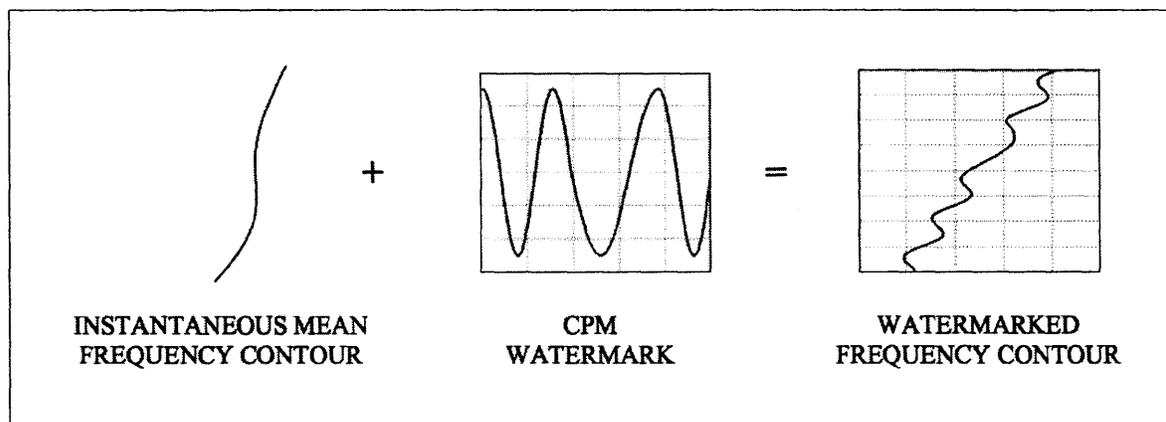
Figure 4-19: Watermarking scheme based on CPM perturbation of the IMF contour
