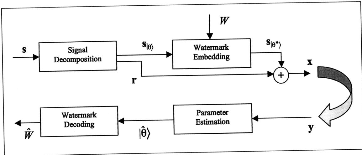
Figure 1-3: Parametric watermarking scheme [38]
