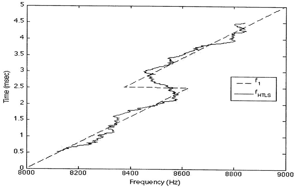
Figure 3-3: HTLS frequency tracking performance for a linear chirp with abrupt frequency shifts (SNR = 5 dB)
