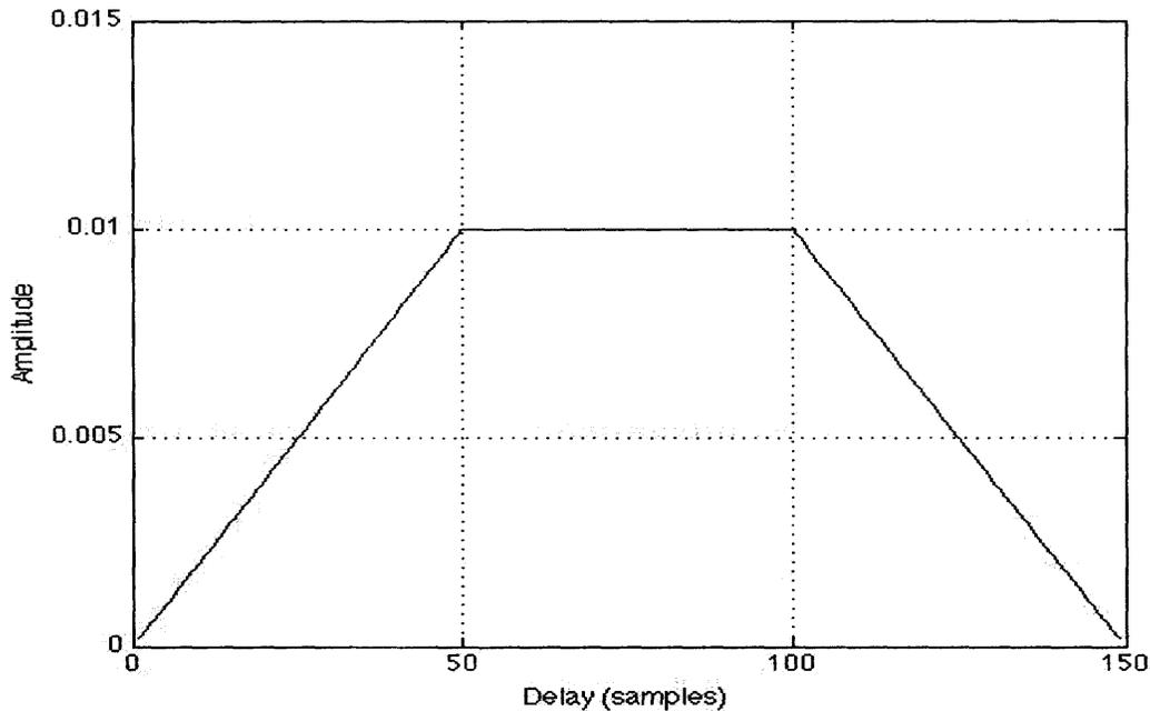
Figure 4-15: Impulse response of moving-average filter
