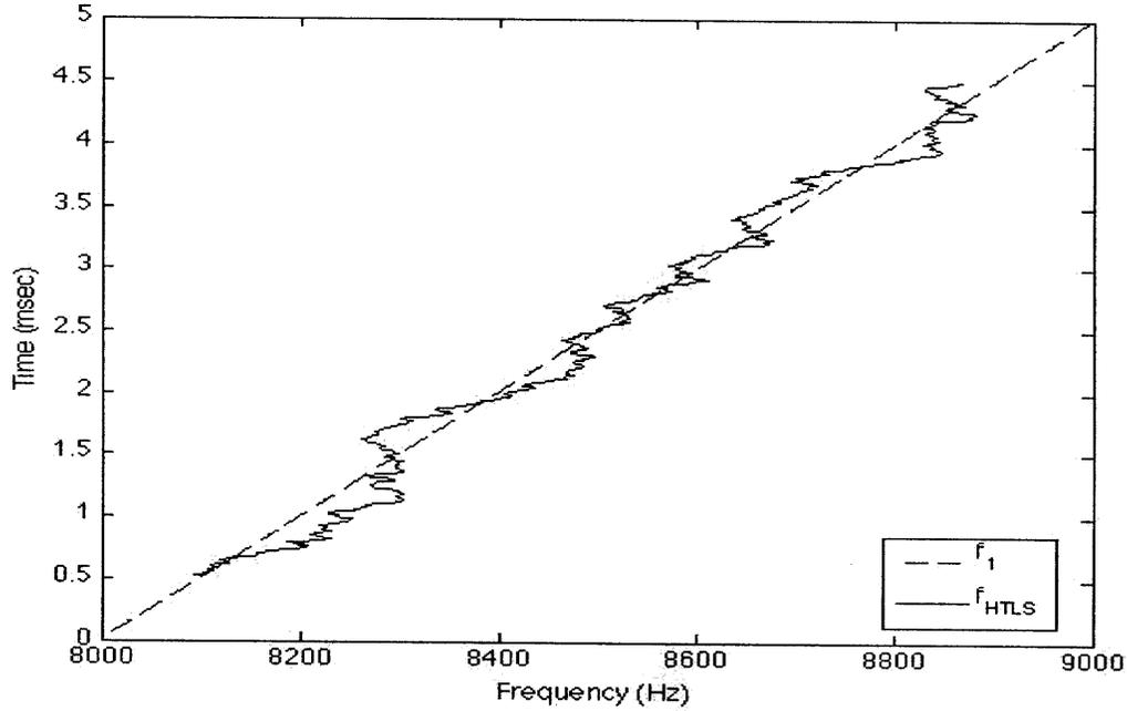
Figure 3-1: HTLS frequency tracking performance for a linear chirp (SNR = 5 dB)
