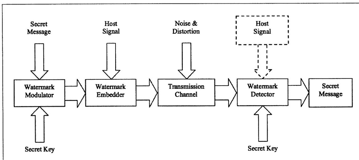
Figure 1-2: Communication model for watermarking [23]
