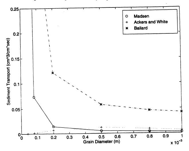
Figure 16. The total sediment transport rate versus sediment diameter for a wave period of 4 sec, an average current velocity of 0.35 m/sec and a maximum wave orbital velocity of 0.35 m/sec.
