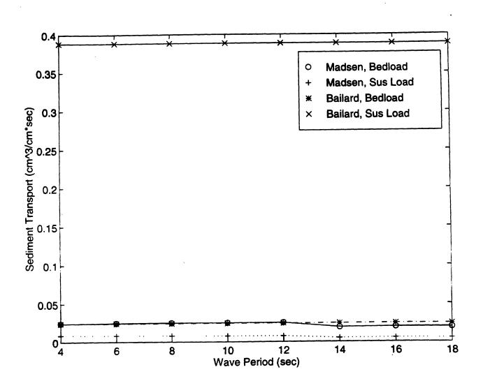
Figure 25. Break down of the total sediment transport rate versus wave period for 0.1 mm diameter sediment, an average current and a maximum wave orbital velocity of 0.35 m/sec.
