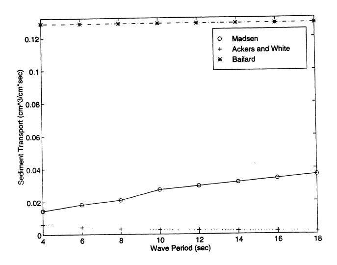
Figure 23. The total sediment transport rate versus wave period, for 0.2 mm diameter sediment, an average current velocity of 0.35 m/sec and a maximum wave orbital velocity of 0.35 m/sec.
