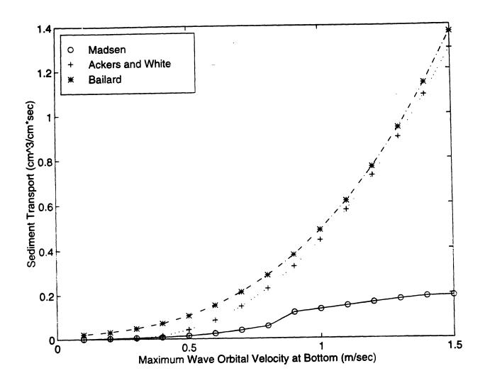
Figure 30. The total sediment transport rate versus maximum wave orbital velocity for a wave period of 8 sec, 0.5 mm diameter sediment, and an average current velocity of 0.35 m/sec.
