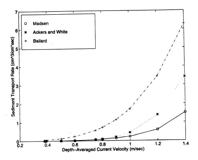
Figure 11. The total sediment transport rate versus depth-averaged current velocity for 0.2 mm diameter sediment and a flow depth of 5 m.
