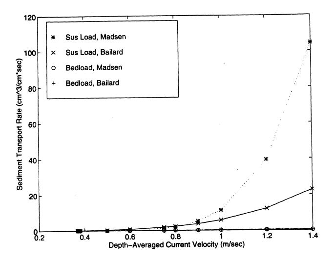
Figure 13. Break down of the total sediment transport rate versus depth-averaged current velocity for the Madsen and Bailard models. Taken for 0.1 mm diameter sediment and 5 m flow depth.
