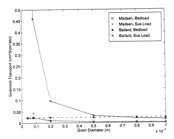
Figure 20. Break down of the total sediment transport rate versus sediment diameter for a wave period of 8 sec, an average current and a maximum wave orbital velocity of 0.35 m/sec.
