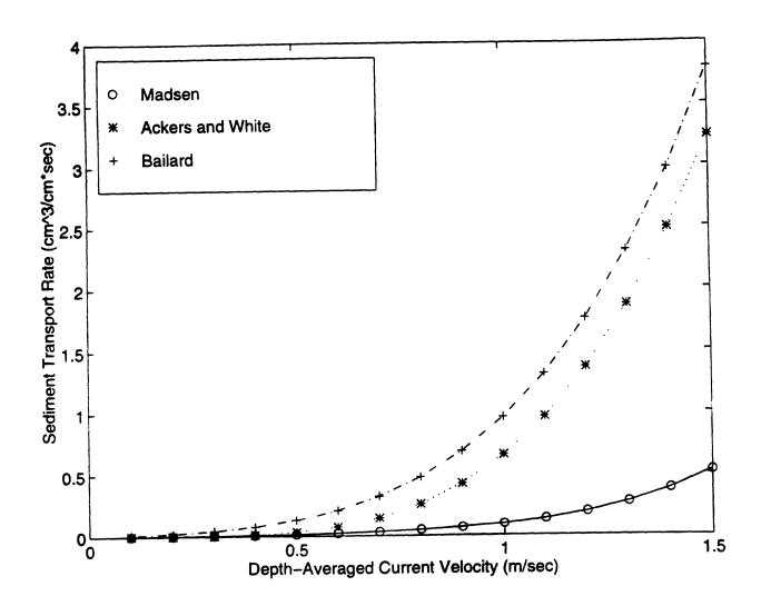
Figure 36. The total sediment transport rate versus the average current velocity for a maximum wave orbital velocity of 0.35 m/sec, a wave period of 8 sec, and 0.5 mm diameter sediment.
