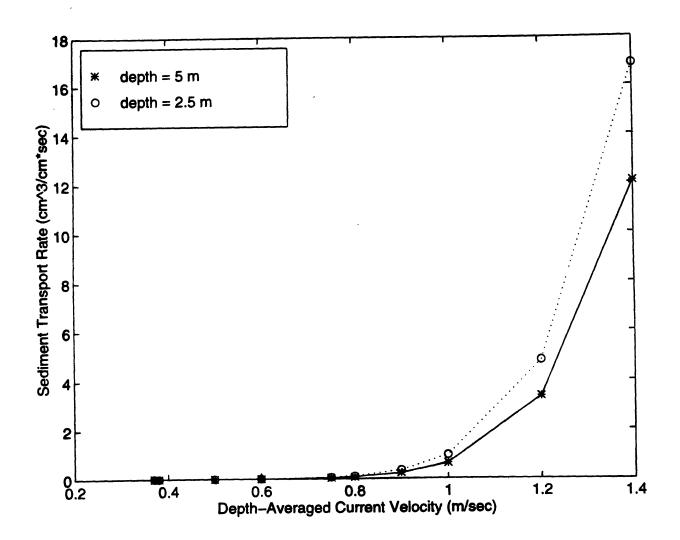
Figure 1. The Ackers and White model, total sediment transport rate versus depth-averaged current velocity for 0.1 mm diameter grains.
