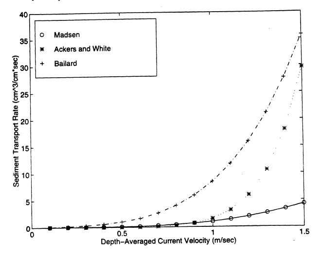
Figure 34. The total sediment transport rate versus the average current velocity for a maximum wave orbital velocity of 0.35 m/sec, a wave period of 8 sec, and 0.1 mm diameter sediment.
