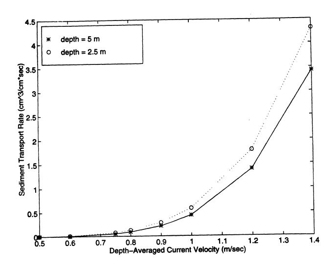
Figure 2. The Ackers and White model, total sediment transport rate versus depth-averaged current velocity for 0.2 mm diameter grains.
