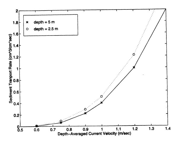
Figure 3. The Ackers and White model, total sediment transport rate versus depth-averaged current velocity for 0.5 mm diameter grains.
