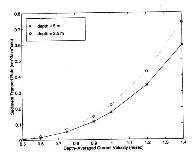
Figure 6. The Madsen model, total sediment transport rate versus depth averaged-current velocity for 0.5 mm diameter grains.
