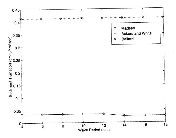
Figure 22. The total sediment transport rate versus wave period, for 0.1 mm diameter sediment, an average current velocity of 0.35 m/sec and a maximum wave orbital velocity of 0.35 m/sec.
