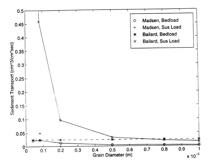
Figure 19. Break down of the total sediment transport rate versus sediment diameter for a wave period of 4 sec, an average current and a maximum wave orbital velocity of 0.35 m/sec.
