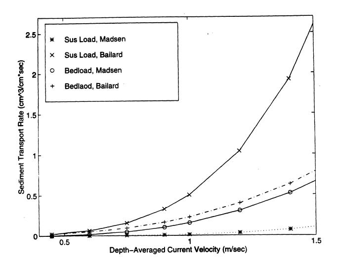
Figure 15. Break down of the total sediment transport rate versus depth-averaged current velocity for the Madsen and Bailard models. Taken for 0.5 mm diameter sediment and 5 m flow depth.
