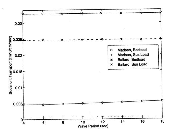
Figure 27. Break down of the total sediment transport rate versus wave period for 0.5 mm diameter sediment, an average current and a maximum wave orbital velocity of 0.35 m/sec.
