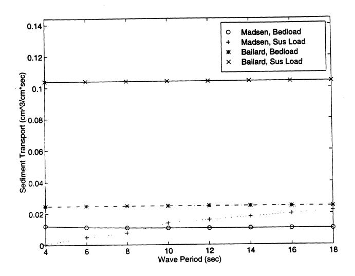
Figure 26. Break down of the total sediment transport rate versus wave period for 0.2 mm diameter sediment, an average current and a maximum wave orbital velocity of 0.35 m/sec.
