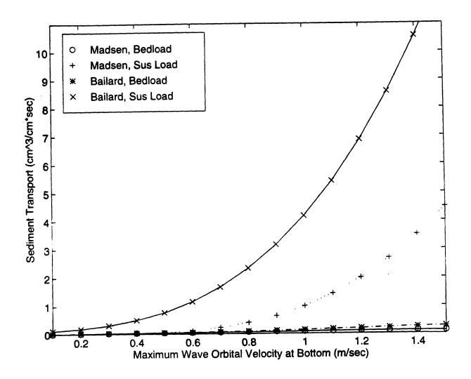
Figure 31. Break down of the sediment transport rate versus maximum wave orbital velocity for a wave period of 8 sec, 0.1 mm diameter sediment, and an average current velocity of 0.35 m/sec.
