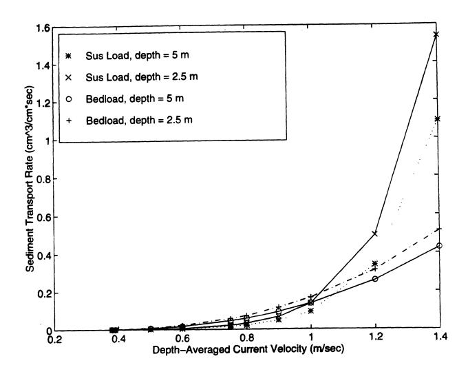
Figure 8. The Madsen model, break down of the total sediment transport rate versus depth-averaged current velocity for 0.2 mm diameter sediment.
