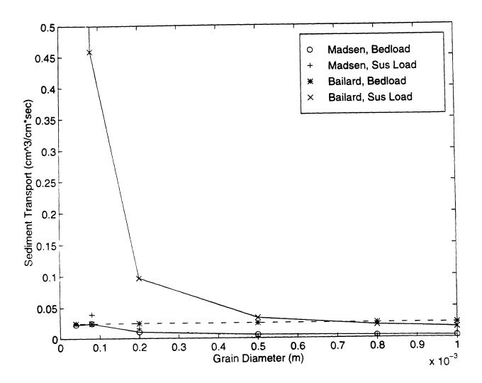
Figure 21. Break down of the total sediment transport rate versus sediment diameter for a wave period of 16 sec, an average current and a maximum wave orbital velocity of 0.35 m/sec.
