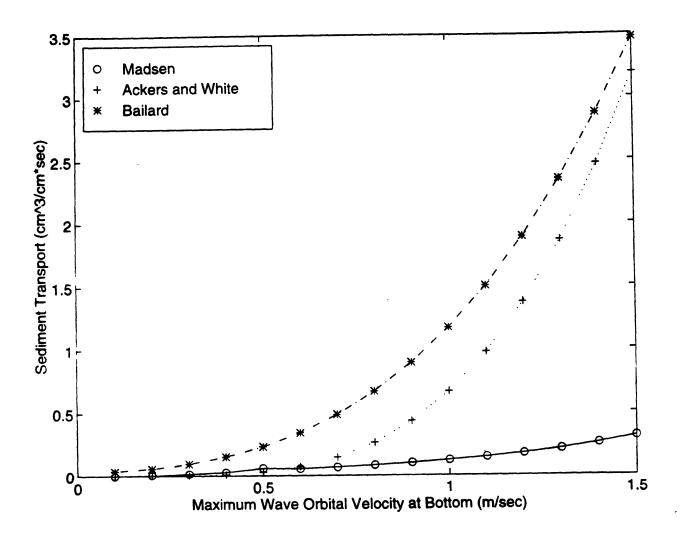
Figure 29. The total sediment transport rate versus maximum wave orbital velocity for a wave period of 8 sec, 0.2 mm diameter sediment, and an average current velocity of 0.35 m/sec.
