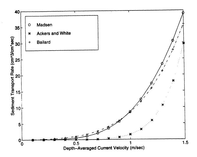
Figure 37. The total sediment transport rate versus the average current velocity for a maximum wave orbital velocity of 0.35 m/sec, a wave period of 8 sec, and 0.1 mm diameter sediment. Same as Figure 34 except that the Madsen resuspension parameter has increased from 0.0002 to 0.002
