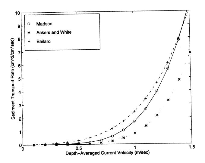
Figure 35. The total sediment transport rate versus the average current velocity for a maximum wave orbital velocity of 0.35 m/sec, a wave period of 8 sec, and 0.2 mm diameter sediment.
