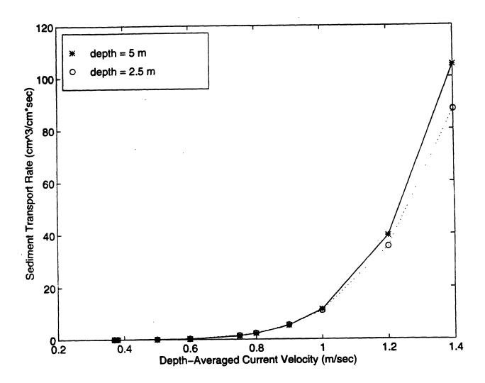
Figure 4. The Madsen model, total sediment transport rate versus depth-averaged current velocity for 0.1 mm diameter grains.
