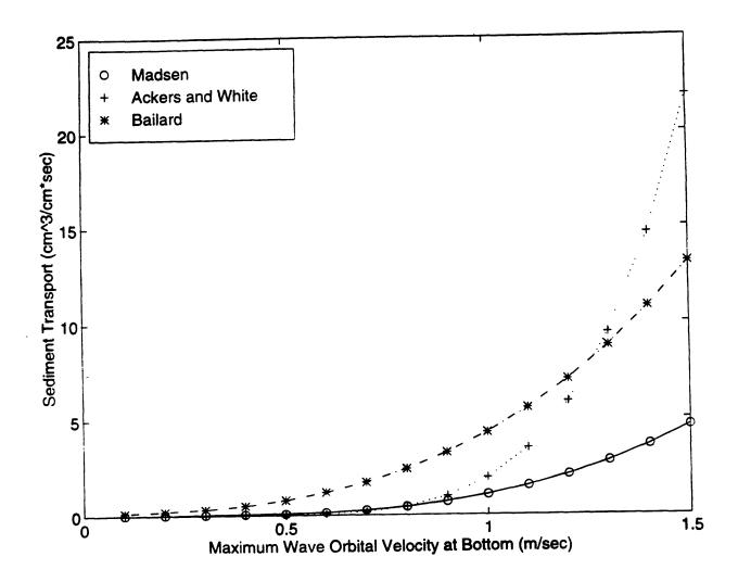
Figure 28. The total sediment transport rate versus maximum wave orbital velocity for a wave period of 8 sec, 0.1 mm diameter sediment, and an average current velocity of 0.35 m/sec.
