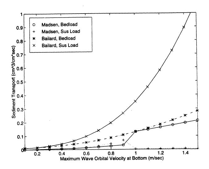
Figure 33. Break down of the sediment transport rate versus maximum wave orbital velocity for a wave period of 8 sec, 0.5 mm diameter sediment, and an average current velocity of 0.35 m/sec.
