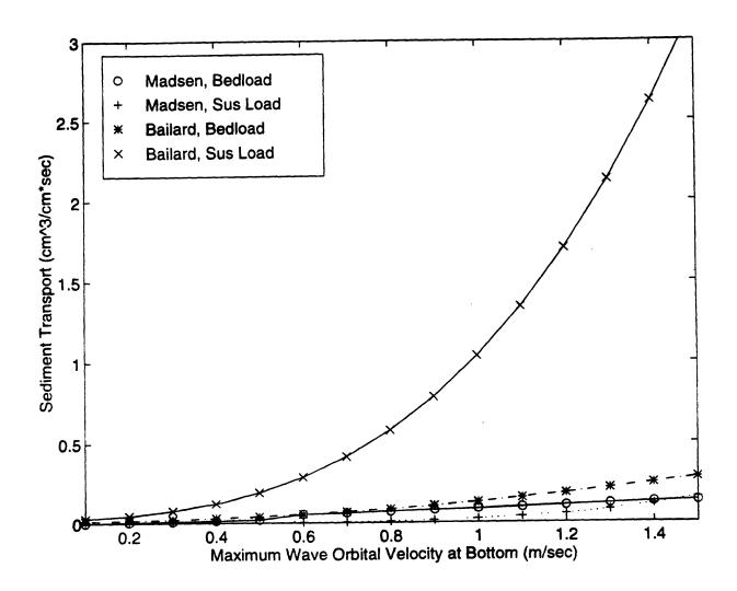
Figure 32. Break down of the sediment transport rate versus maximum wave orbital velocity for a wave period of 8 sec, 0.2 mm diameter sediment, and an average current velocity of 0.35 m/sec.
