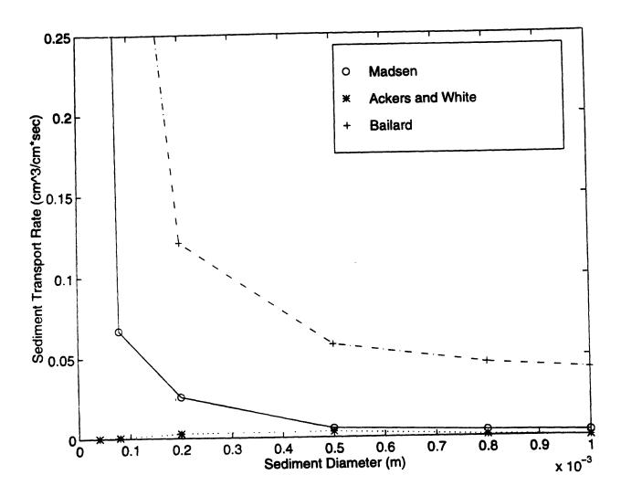
Figure 18. The total sediment transport rate versus sediment diameter for a wave period of 16 sec, an average current velocity of 0.35 m/sec and a maximum wave orbital velocity of 0.35 m/sec.
