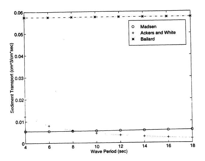
Figure 24. The total sediment transport rate versus wave period, for 0.5 mm diameter sediment, an average current velocity of 0.35 m/sec and a maximum wave orbital velocity of 0.35 m/sec.
