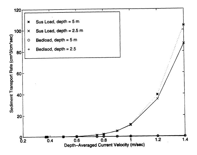
Figure 7. The Madsen model, break down of the total sediment transport rate versus depth-averaged current velocity for 0.1 mm diameter sediment.
