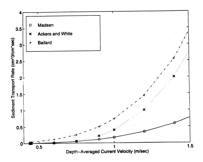
Figure 12. The total sediment transport rate versus depth-averaged current velocity for 0.5 mm diameter sediment and a flow depth of 5 m.
