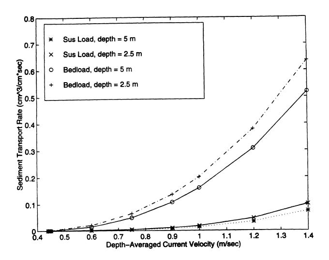
Figure 9. The Madsen model, break down of the total sediment transport rate versus depth-averaged current velocity for 0.5 mm diameter sediment.
