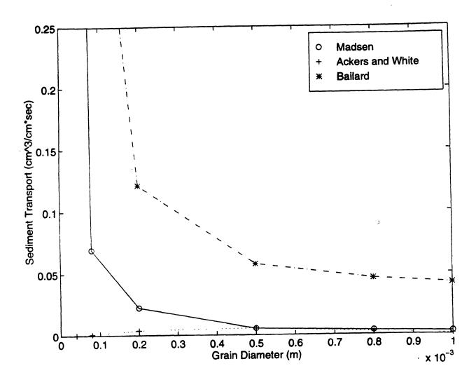
Figure 17. The total sediment transport rate versus sediment diameter for a wave period of 8 sec, an average current velocity of 0.35 m/sec and a maximum wave orbital velocity of 0.35 m/sec.
