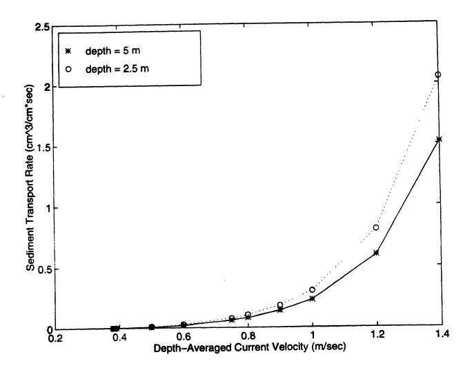
Figure 5. The Madsen model, total sediment transport rate versus depth averaged-current velocity for 0.2 mm diameter grains.
