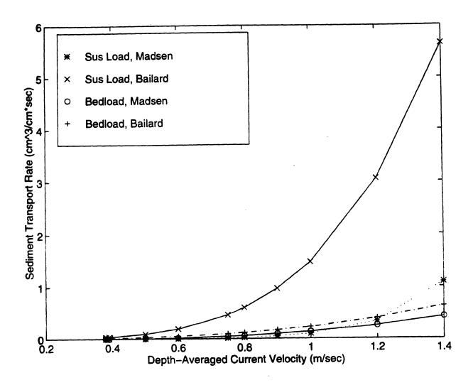
Figure 14. Break down of the total sediment transport rate versus depth-averaged current velocity for the Madsen and Bailard models. Taken for 0.2 mm diameter sediment and 5 m flow depth.
