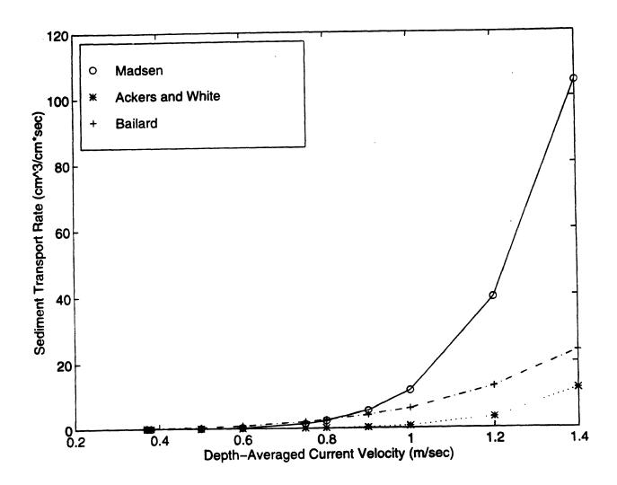
Figure 10. The total sediment transport rate versus depth-averaged current velocity for 0.1 mm diameter sediment and a flow depth of 5 m.
