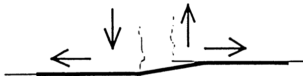
Figure 1.3: Peeling of the Laminate Due to Shear Cracking
