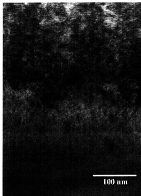
Figure 6.6 – X-TEM image depicting a DMA graded buffer constructed with InP and GaP layers. The GaAs substrate is at the bottom.
