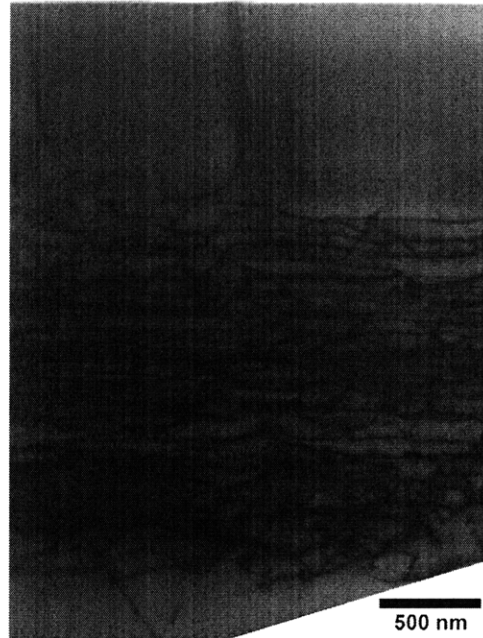
Figure 3.4 – X-TEM of GB3, an InGaAs graded buffer graded at a rate of 1.39% misfit/ \mu\text{m} . Note the dislocation contrast that abruptly turns from a misfit into a thread when its glide is impeded at a phase-separated region.
