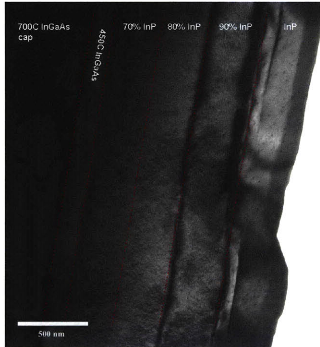
Figure 6.11 – X-TEM image of DMAGB4, a hybrid InGaAs random-alloy graded buffer + DMA graded buffer.
