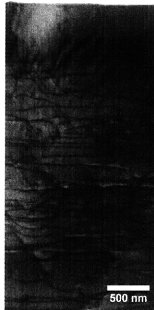
Figure 3.5 – X-TEM of graded buffer GB6. Periodic contrast characteristic of phase separation is clearly visible near the top of the graded buffer.
