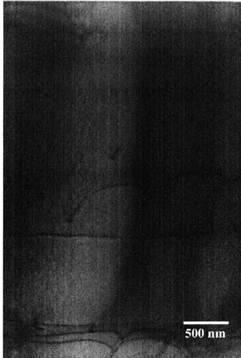
Figure 5.2 – X-TEM image of HBT_1 that was re-grown on an \text{In}_{0.295}\text{Ga}_{0.705}\text{As} graded buffer.
