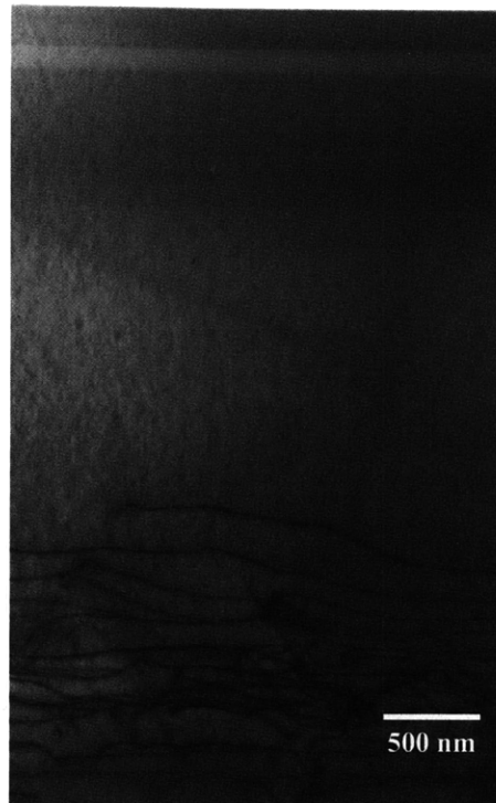
Figure 5.7 – X-TEM image of HBT_3 that was grown continuously together with an \text{In}_{0.305}\text{Ga}_{0.695}\text{As} graded buffer.
