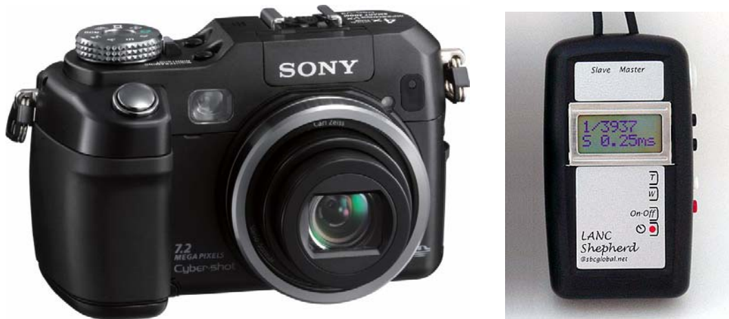
Figure 3.5 Sony V3 digital camera (left) and Shepherd LANC controller (right) (Right photograph provided by Berezin Stereo Photography Products, http://www.berezin.com/3d/ )
