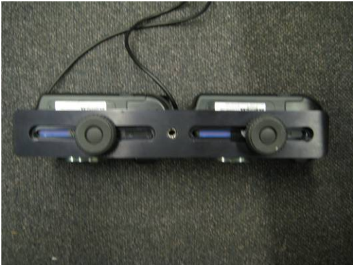
Both cameras aligned and secured
