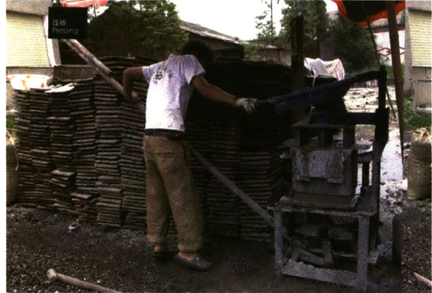
a common brick-pressing machine uses human power and leverage to create bricks
