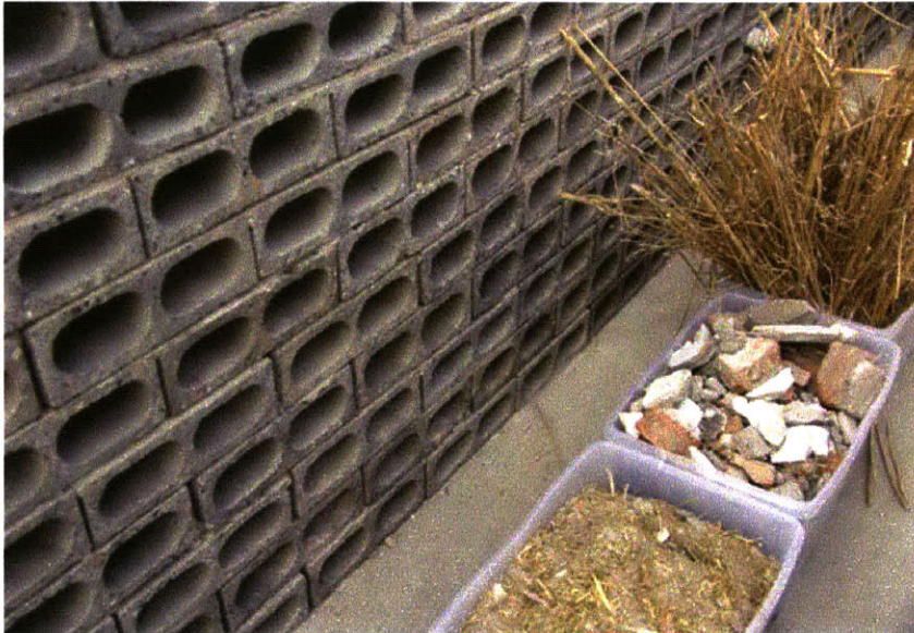
wheat branches, cement and recycled aggregate form the basic ingredients of the "rebirth brick"
