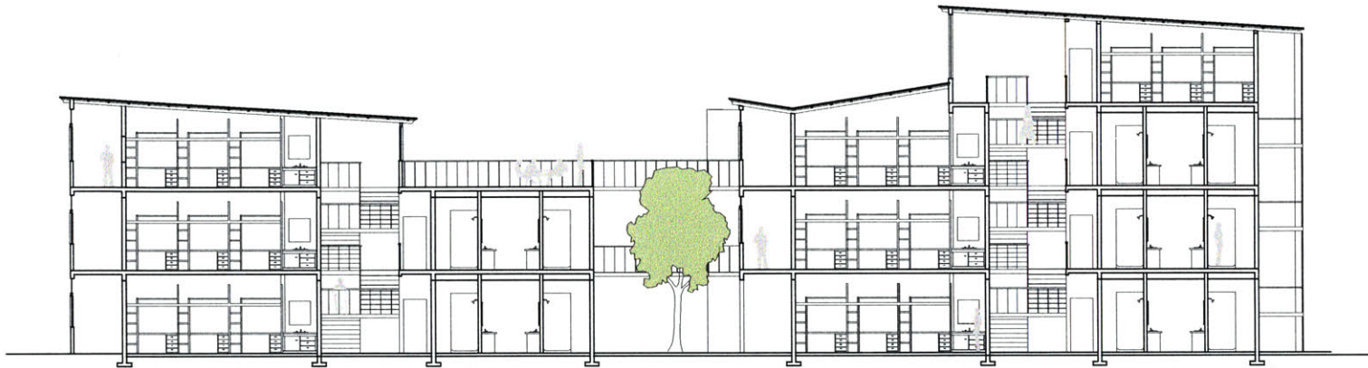
dormitory section through roof deck and courtyard
