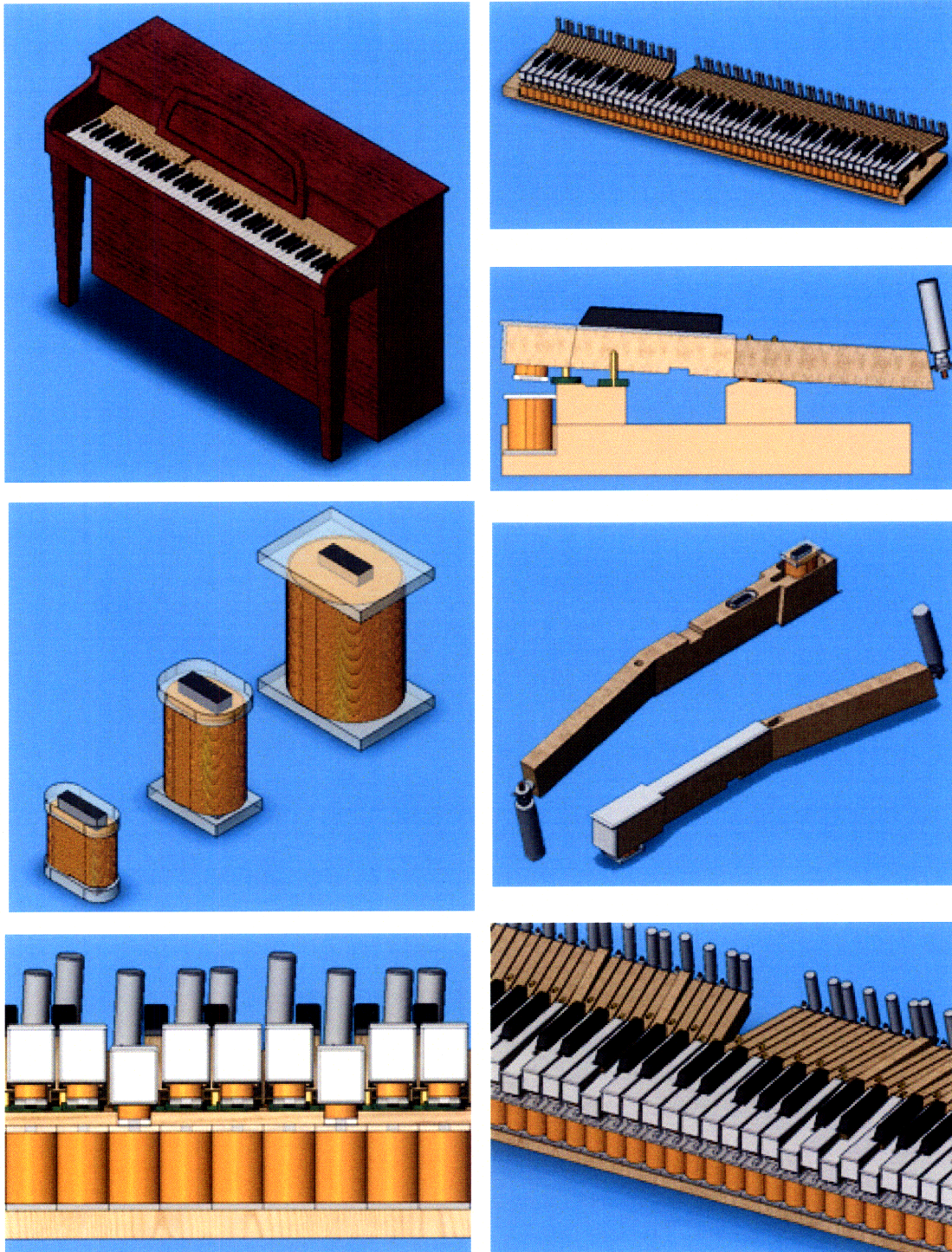
Figure 5-4: SolidWorks model of MagKeyS Trainer Piano. The full keyboard, including electromagnets, alignment pins and counterweights, were modeled in SolidWorks. All images © 2008 Jennifer Doyle.
