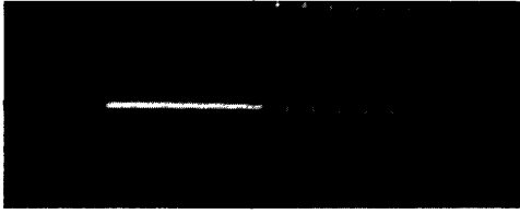
(a) Clamp to negative peak of 500 cycle sinusoidal input.
