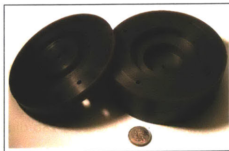
Figure 4-29: Wax Mold Used to Create an Elastic Holder
