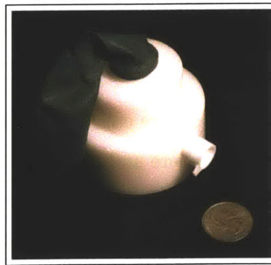
Figure 4-4: Press-Fit Delrin Support
