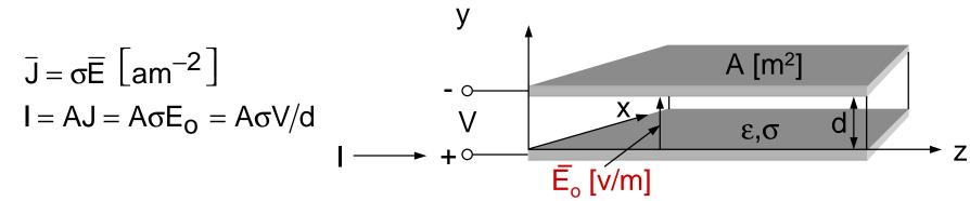
Resistance R: $R = V/I = d/A\sigma$ Resistors in Series: $R_{eq} = R_1 + R_2$  $R_{eq} = (V_1 + V_2)/I$ Resistors in Parallel: $1/R_{eq} = 1/R_1 + 1/R_2$  $1/R_{eq} = (I_1 + I_2)/V$
