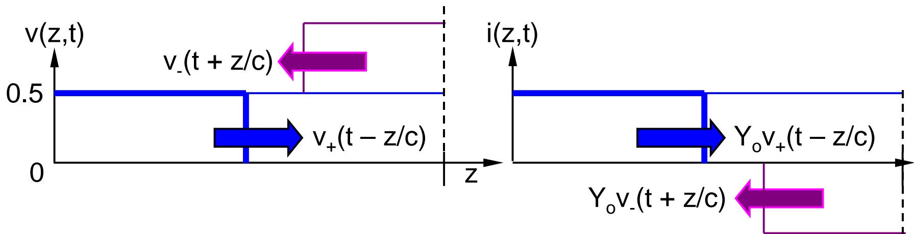
$$v(z,t) = v_+(t - z/c) + v_-(t + z/c) = 0.5[u_{-1}(t - z/c) + u_{-1}(t + z/c - 2W/c)]$$
