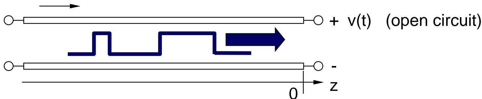
Since:  $i(z,t) = Y_o[v_+(t - z/c) - v_-(t + z/c)] = 0$  at  $z = 0$
