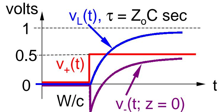
$$i(z,t) = Y_o[v_+(t - z/c) - v_-(t + z/c)]$$
