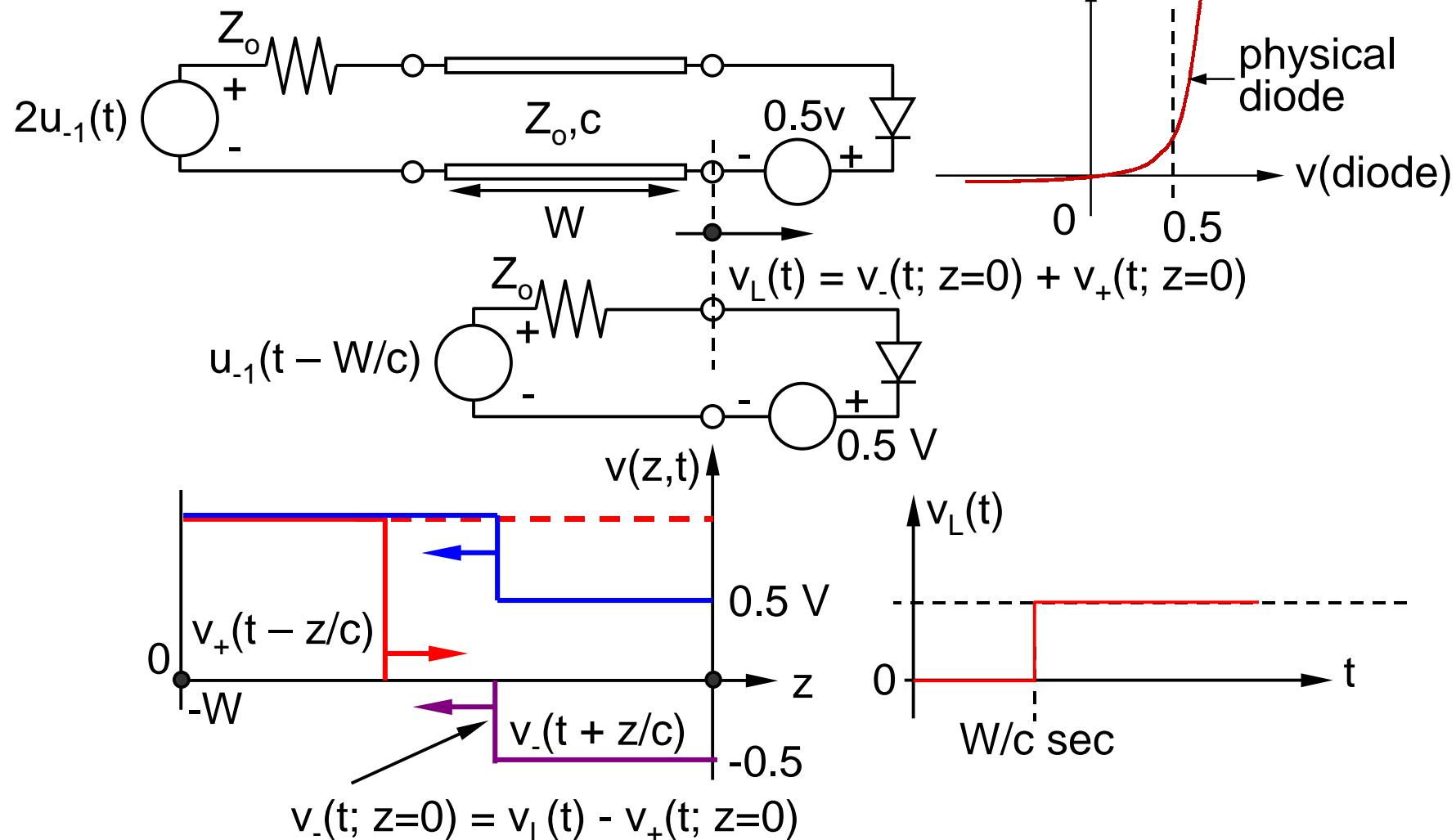
$$v(z, t) = v_+(t - z/c) + v_-(t + z/c)$$
