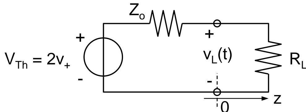
$$v_L(t) = V_{Th}R_L/(R_L + Z_o)$$
