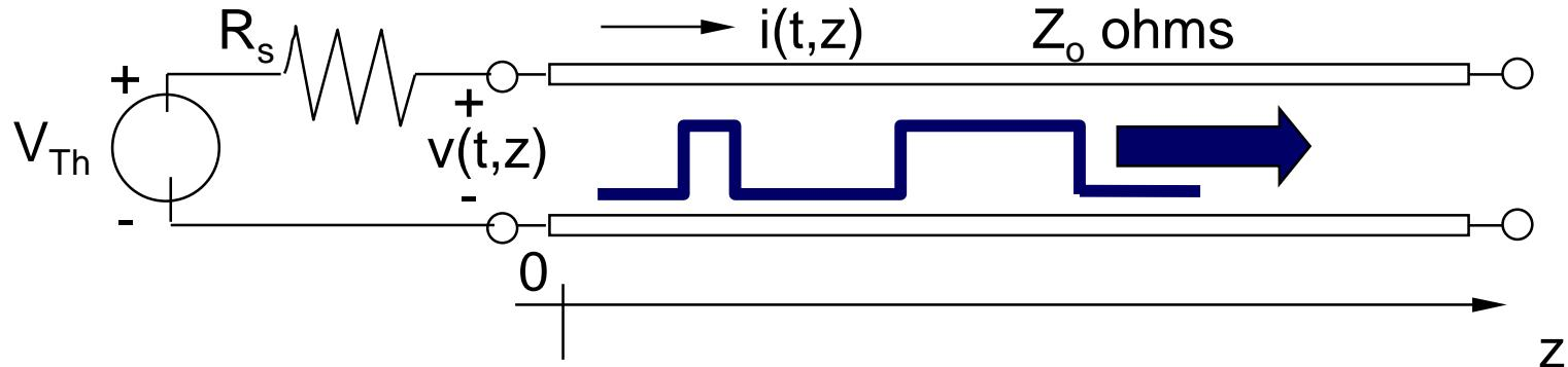
$$v(z,t) = v_+(t - z/c) + v_-(t + z/c)$$
