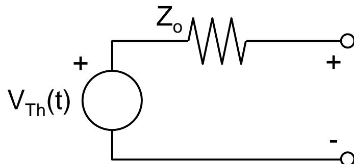
$$v_{\text{open circuit}}(t) = 2v_+(t, z=0)$$
