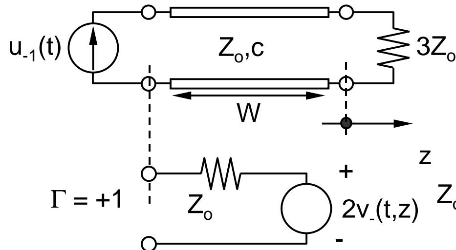
$$\begin{aligned}\Gamma &= (R_L - Z_0)/(R_L + Z_0) \\ &= (3 - 1)/(3+1) = 1/2\end{aligned}$$
