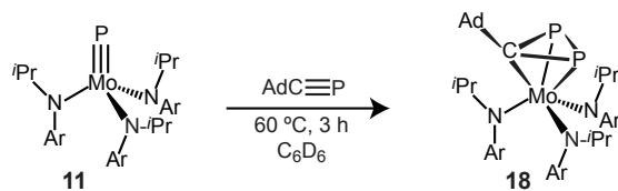
Scheme 1.14. The reaction of AdCP with 11 proceeds analogously to the putative P 2 trapping reaction to afford a cyclo -CP 2 complex ( 18 ).
