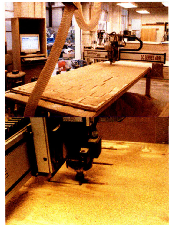
CNC router cutting out building components (Image: http://ddf.mit.edu/projects/CABIN/cabin_full_cnc.html )
