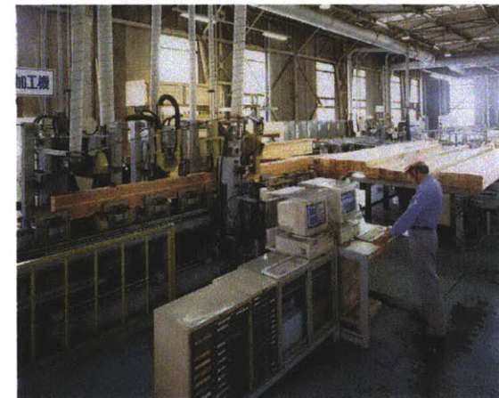
Sekisui House highly automated production line making timber framing (image by Sekisui House).
