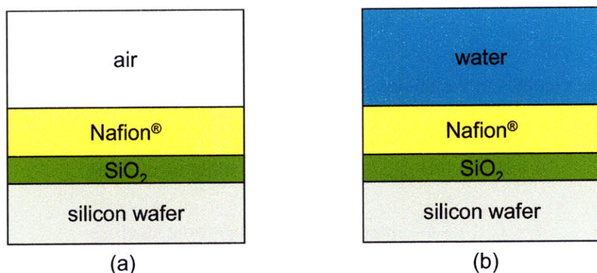
Figure 22. Layer models used for ellipsometry. Nafion ® thin films are exposed to (a) air and (b) liquid water.
