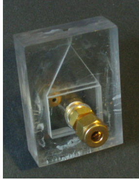
Figure 3-2: Example of Fabricated Nozzle
