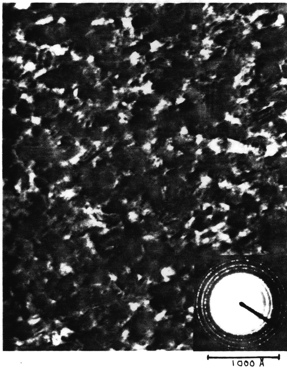
Figure 3.3: Transmission electron micrograph and transmission electron diffraction pattern for polycrystalline as-deposited Ge film on thermal \text{SiO}_2 after deposition at 400^\circ\text{C} .
