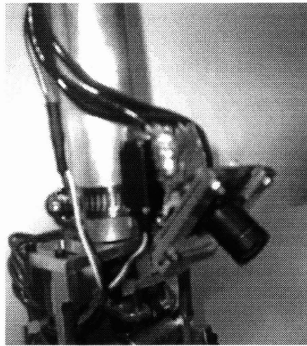
Figure 3-9: The “eye-on-hand” camera
