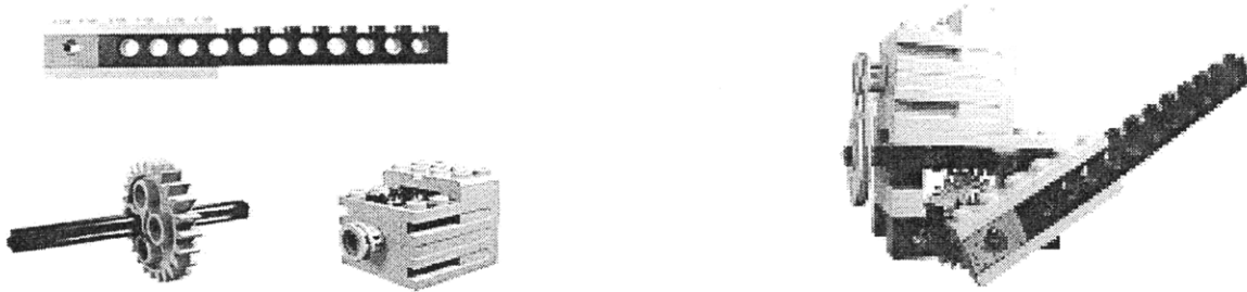
Figure 3-2 Relationships in a physical model. The components on the left can be associated with various functions. As unique components however, it is unlikely that anyone would identify the intended configuration on the right. The integrated view allows us to understand how these components combine to provide a larger function.
