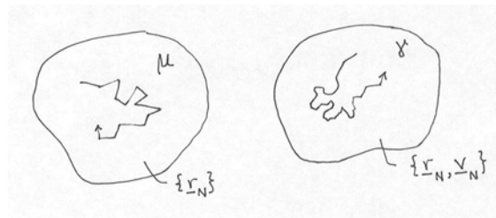
Fig. 2. Schematic depicting the evolution of the same N -particle system in the 3-N dimensional configurational space ( \mu ) as sampled by MC, and in the 6-N dimensional phase space ( \gamma ) sampled by MD. In each case, the sampling results in a trajectory in the
