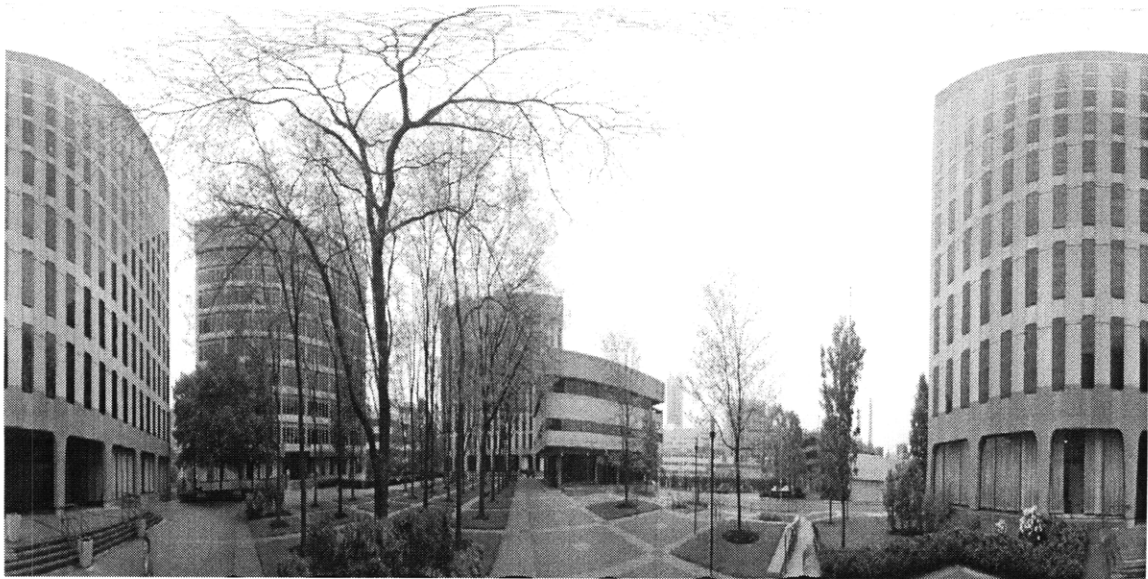
Figure 5-2: A spherical mosaic, using images acquired with Argus. The rectangular picture was produced by environment mapping the hemisphere onto a cylinder, and unrolling the cylinder. Mosaic courtesy of Neel Master and Satyan Coorg.
