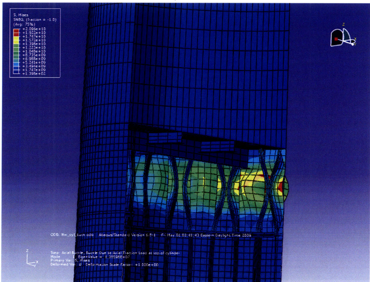
Figure 8.11-ABAQUS Rendering of Mises Stresses for Axial Buckle Load
