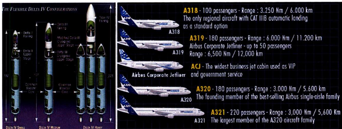
**Figure 2: Examples for aerospace systems portfolios where the systems exhibit identical externally delivered functions: Delta IV launch vehicle family (left); A320 commercial aircraft family (right)**
