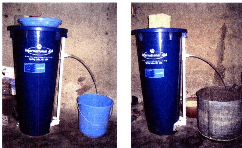
Figure 7-5 BSF filtrate collection vessels: a) plastic bucket with lid and b) garawa
