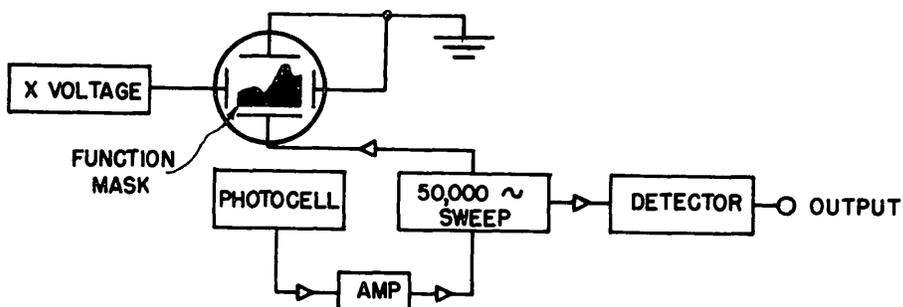
Figure 1 Mark II double-sweep function generator
