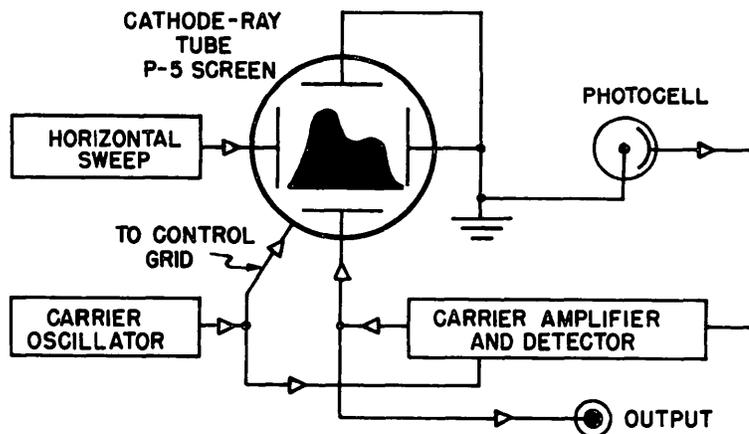
Figure 2 A continuous-tracking function generator
