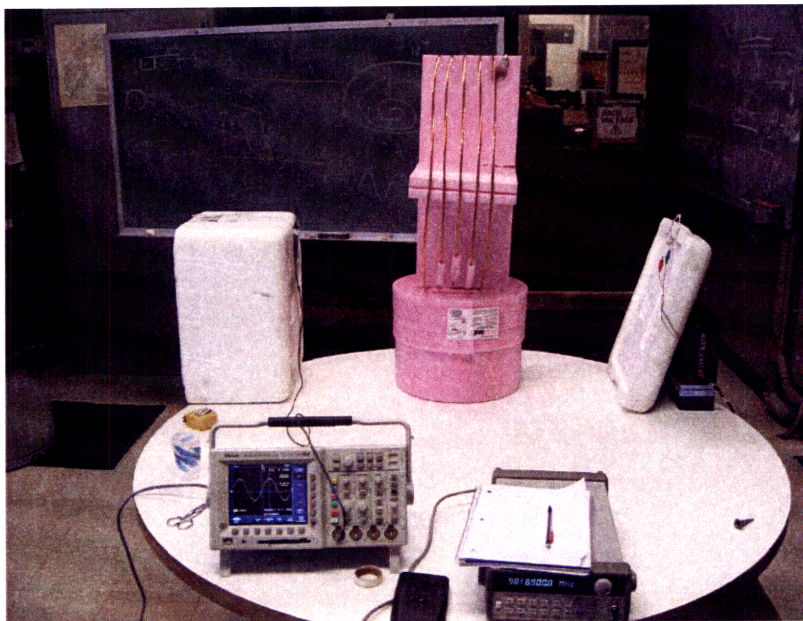
Figure 4-4: Photograph of the setup for measuring coil Q . Photo provided by Andre Kurs.
