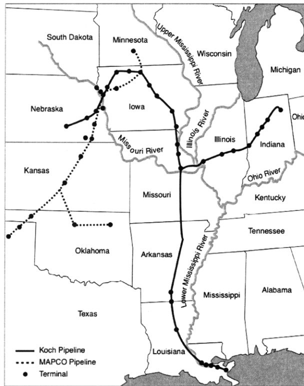
Figure 2: Ammonia Pipelines (the owners have changed)
