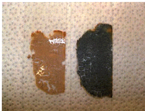
Figure 34. Change in polyelectrolyte complex color with hydrogen cyanide
