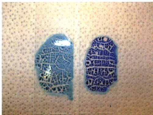
Figure 29. Change in polyelectrolyte complex color with ammonia
