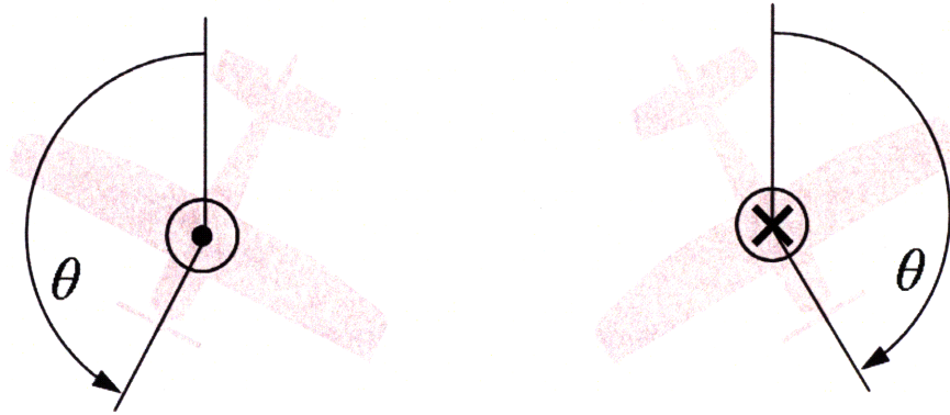
(a) Positive rotation with axis pointing out of the page (b) Positive rotation with axis pointing into the page
