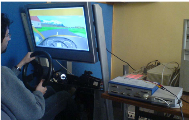
Fig. 19. Hardware-in-the-loop test setup.
