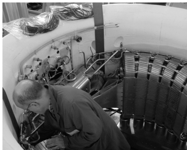
Fig. 9. The magnet being fitted into the bore of the helium vessel.
