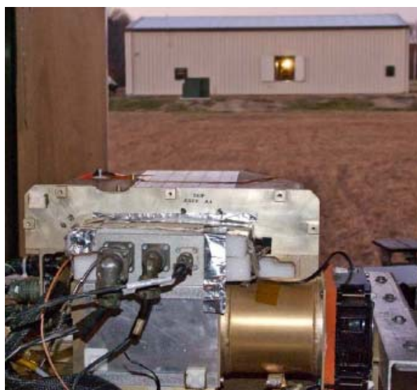
Figure 5: A photograph of the lidar sensor head in the foreground with the Vortex Chamber building in the far ground or out-range.
