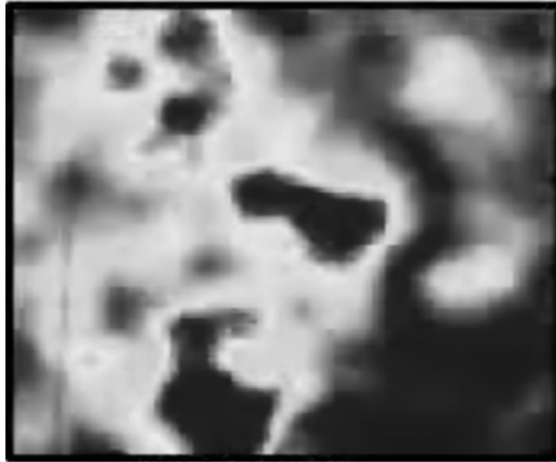
Fig. 4. Measured intensity pattern over an 8"x 8" area. The characteristic size of the scintillation features is comparable to the separation between the receiver apertures.
