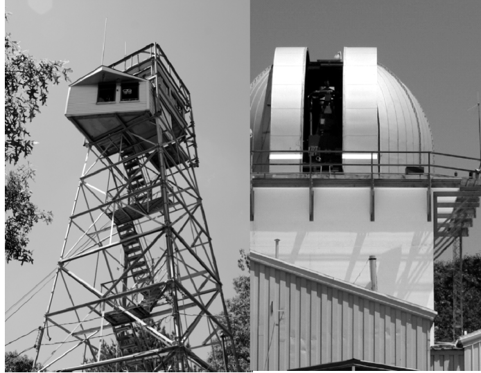
Fig. 1. Fire tower housing the transmitter and telescope dome housing the receiver. These platforms were separated by a distance of 5.4 km.
