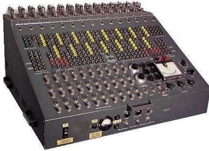
Figure 1-3: An analog electronic computer, the Heathkit H1 from 1956. Image source: http://www.technikum29.de/ .
