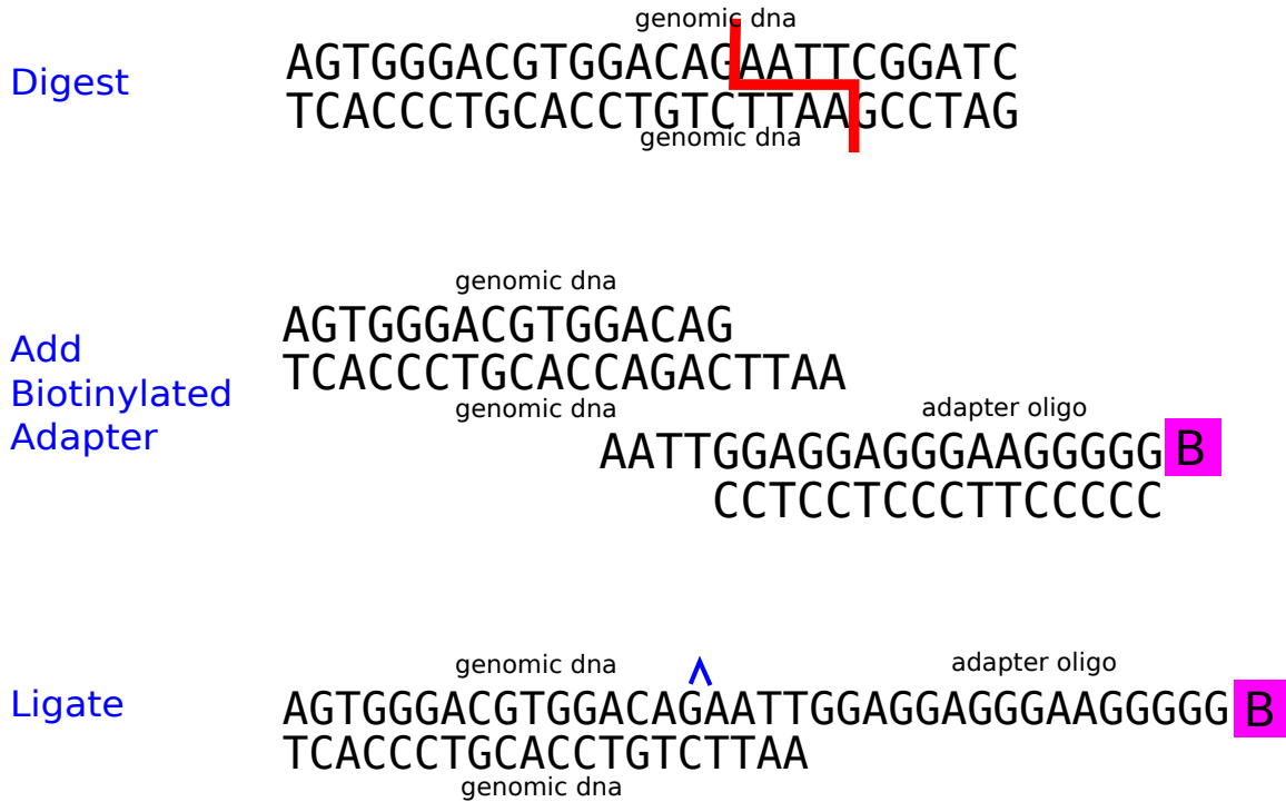
Figure 3-3: The digestion and ligation steps of the Ruler Array protocol attach an adapter molecule to specific genomic loci. The adapter is biotinylated such that the ligated material can be separated from the unligated material.
