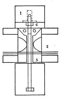
b. VERTICAL SECTION OF JOINT BETWEEN WALL ELEMENTS AND FLOOR SLAB. NEY: 1 WALL ELEMENTS 2. FLOOR SLAB, 3 GUIDING AND HOISTING BOLT, 4. ADJUSTABLE NUT, 5. ROOFING FELT UNDER TWO BEARING PROJECTIONS, 6. GROUTING WITH CEMENT MORTAR, 7. GUIDE HOLE IN WALL ELEMENT
