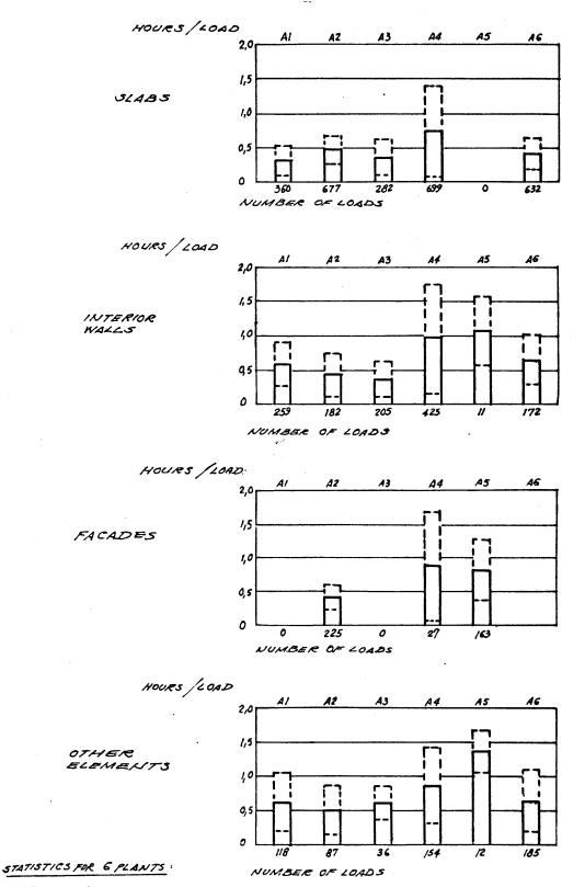
THE FOR LOADING, MEANS AND DISPERSION FOR FLOORS, INTERNAL AND EXTERNAL WALLS AND OTHER MINDS OF UNITS THE CONTINUOUS LINE - THE MEAN, THE BROKEN LINE - A STANDARD DEVIATION THE DISPERSION IS CALCULATED FOR THE MEAN OF THE TIME PER HAUL DURING ONE DAY FO EVERY VEHICLE USED.
