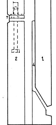
C. VERTICAL SECTION OF JOINT BETWEEN STARCASE FACADE ELEMENTS. KEY: I EXTERNAL CONCRETE, Z. INTERNAL CONCRETE, B.INSULATION A. FLASTIC FOIL, S. GUIDING AND MOISTING BOLT, G. FILLING, T.CEMENT MORTAR JOINT
