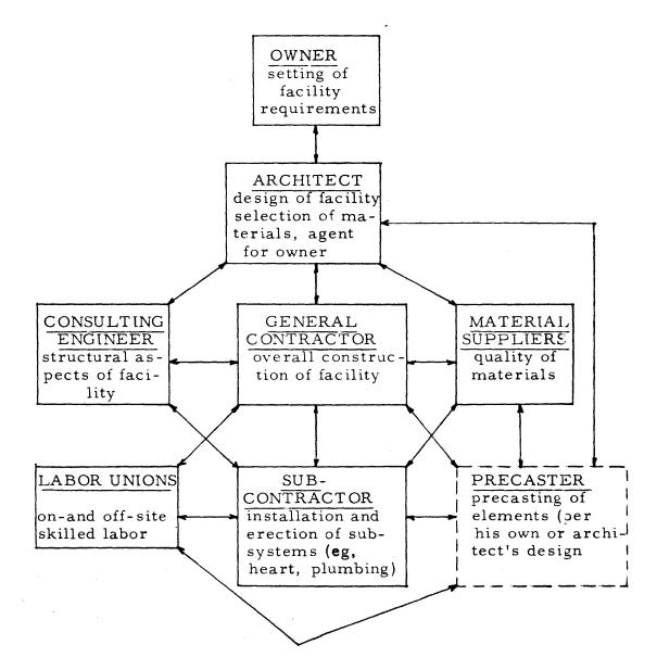
NOTE: The Actors and their interactions in the precast concrete industry. Arrows indicate the flow of information and control.
