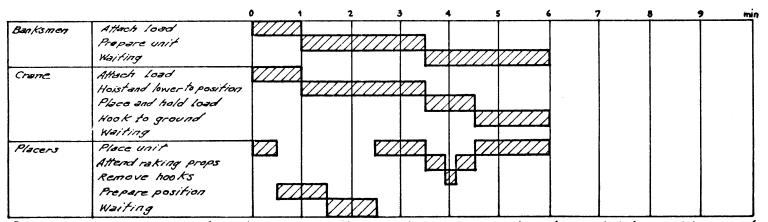
Potential cycle time per panel which could be obtained if chane were released immediately panel is secured
