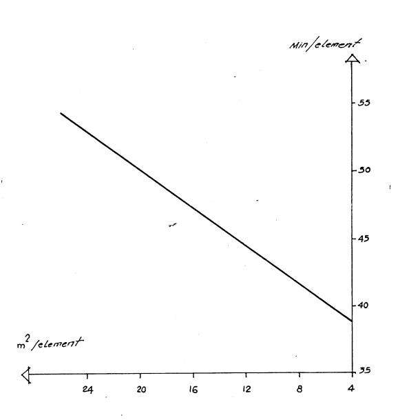
PREPARATION OF BATTERY= STEEL PLACING
