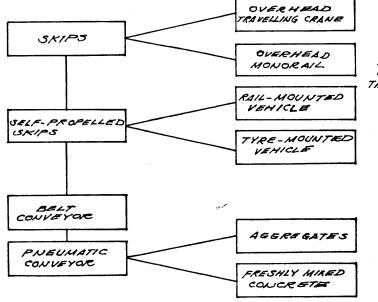
PSSIBILITIES FOR TRANSFORT OF FRESH CONCRETE WITHIN THE PRECASTING WORKS
