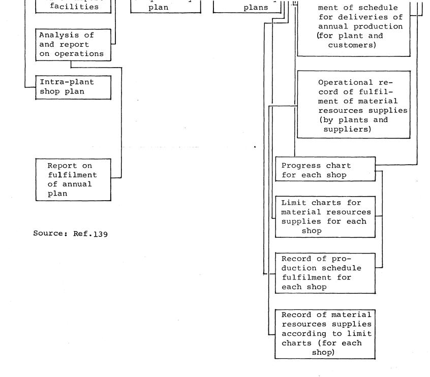
Schematic diagram of automated planning and production management system for a precast reinforced concrete plant.
