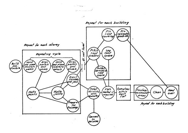
SEQUENCE OF OPERATIONS FOR A BLOCK OF FLATS WITH STAIRWELL ACCESS
