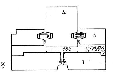
3. NORIZONITAL SECTION BETWEEN FACADE AND WALL ELEMENTS . KEY : 1 EXTERNAL CONCRETE, 2. INSULATION, 3. INTERNAL CONCRETE, 4. WALL ELEMENT, 5. THE -LUE, 6. FILLING, 7. RAIN PROTECTION
