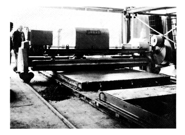
Figure: 36 Finishing Screed passing over a compacted wall element.
