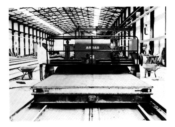
Figure: 33 ARBAU-Finishing Screed floating a two-piece element.
