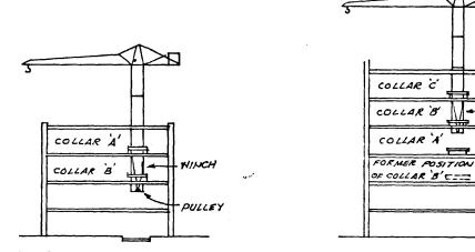
FIG.3 (LEFT) CEANE DETACHED FROM FOUNDATIONS, LIFTED THROUGH COLLDRS WITH HAND WINCH AND REFIXED
