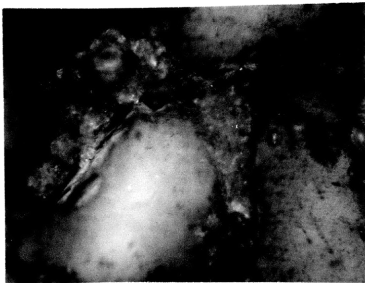
Fig. 25e (Specimen 2) Microcracks and segregation at interface in this post straining parallel section. (220X)
