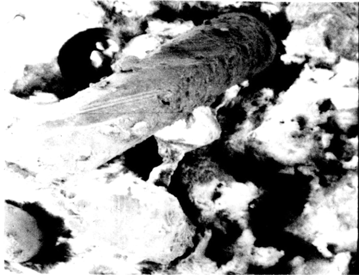
Fig. 29a (Specimen 13) Fracture surface view showing irregularity of crack in three dimensional space. (SEM at 60X)
