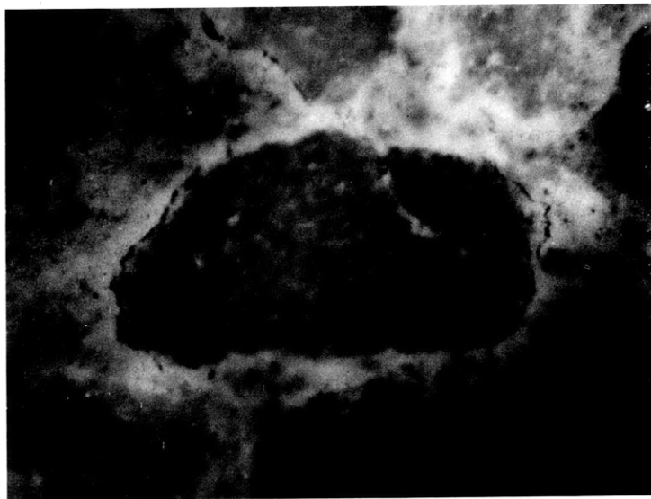
Fig. 25b (Specimen 5) Poor paste aggregate interface bond causes crack to surround this particle as specimen fractured all across. (110X)
