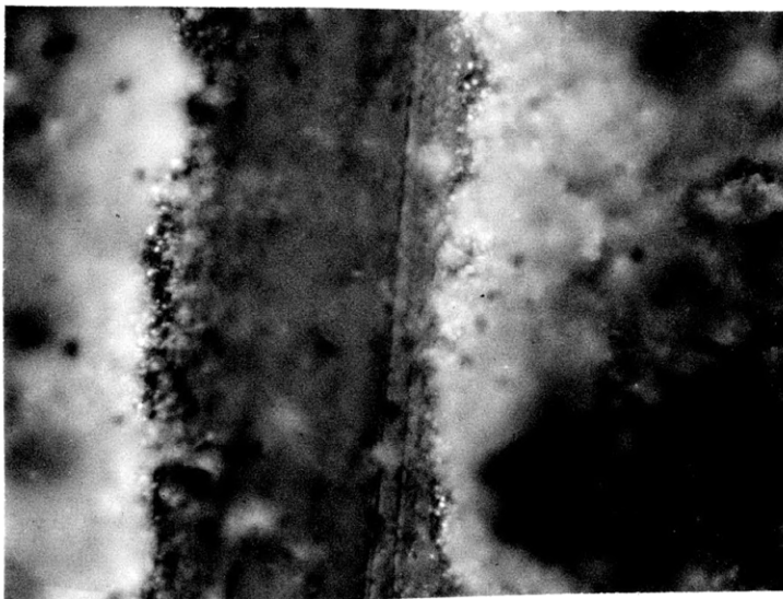
Fig. 26b (Specimen 23) Note excellent bonding here where surface is polished away from wire. (220X)
