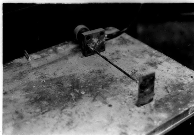
Fig. 12b Vibrating Table and Pneumatic Compacting Tool.
