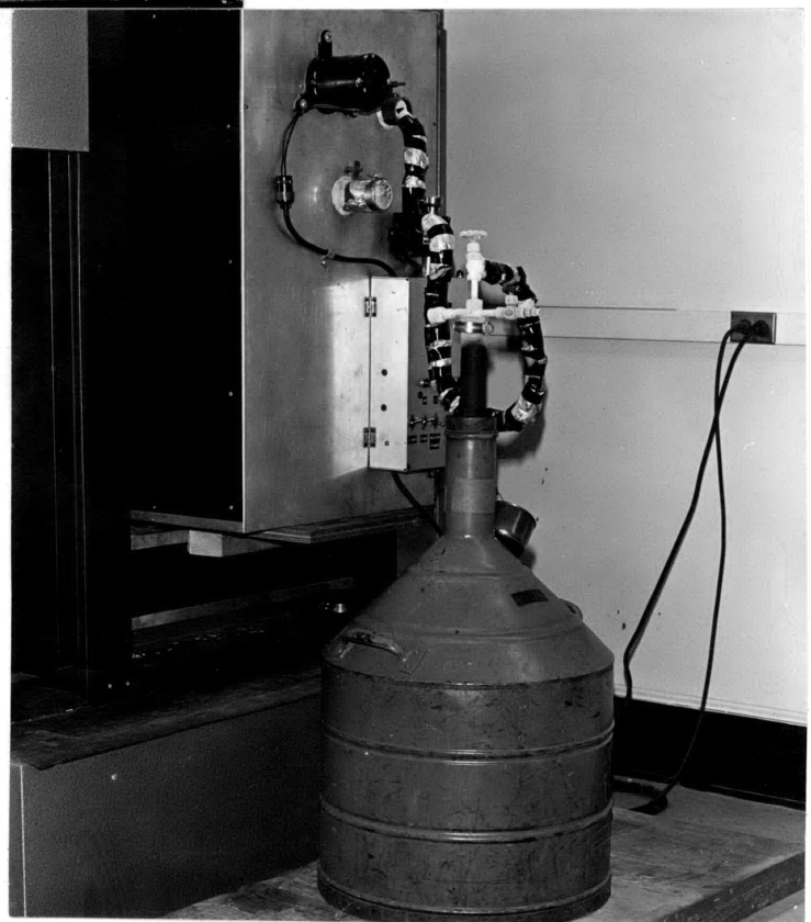
Figure 6 - Apparatus for Testing Beams in Silicone Oil
