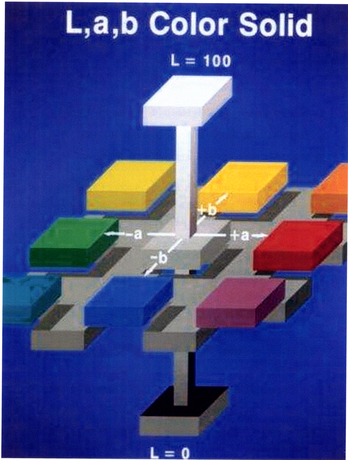
Figure 4-1: Color Quality Chart: L,a,b are the three variables which quantify and characterize indigo color quality
